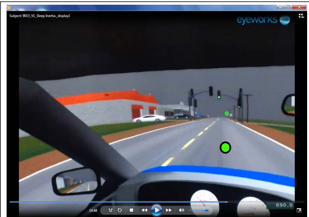
Figure 10. Integration of eye tracking with driving simulator.
