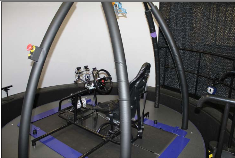
Figure 2. NHRC custom-designed driving simulator.
