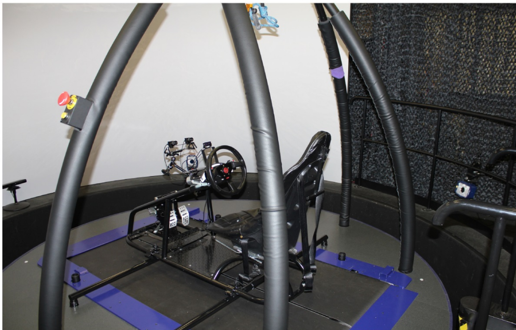
DRIVING SIMULATOR SECURED ON MOTION PLATFORM
