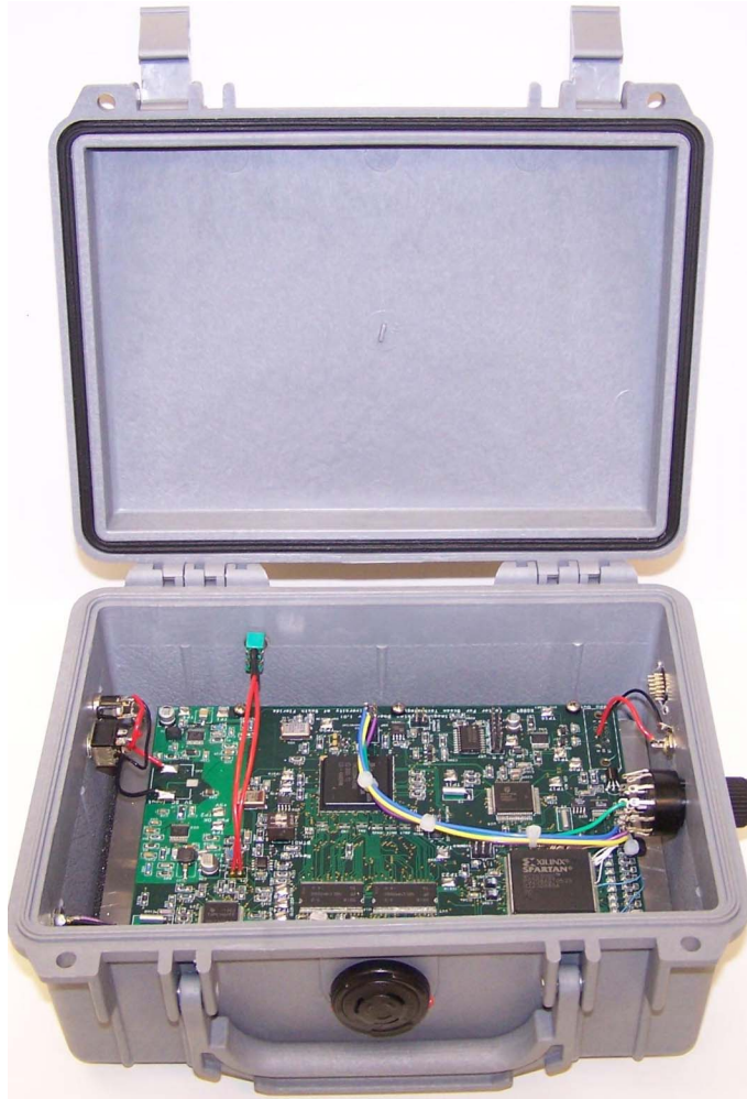
Figure 1: A photo of the circuit board mounted temporarily in a plastic case for protection. [The circuit board measures roughly 5x7 inches and is mounted in a plastic case measuring 6x8x 4 inches. The circuit board is densely populated with several hundred surface mount components].
