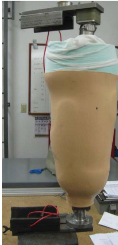
Figure 2.6. Socket test setup (WillowWood, 2012)
