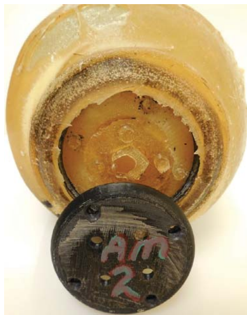
Figure 2.8. Failed distal adapter on tested AM socket
