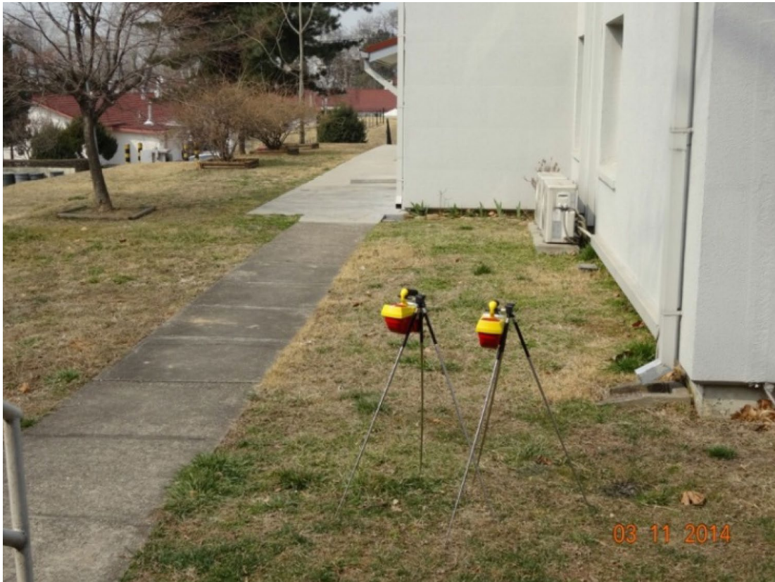
Figure C2. Side-by-side fluke 451 ion chambers mounted on tripods Source: DoD OIG
