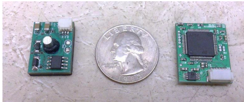
Figure 1: Complete cumulative injury-energy sensing package (CBI-ESP), final delivery
