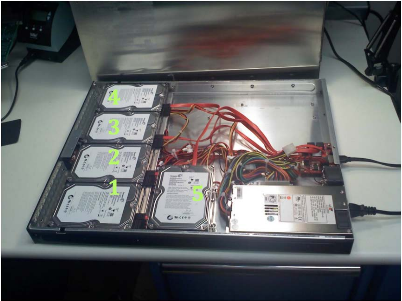
Figure 2. The data recorder storage unit with the case open to expose the 5 drives.
