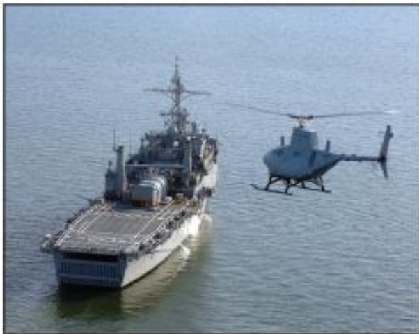
ATLANTIC OCEAN (January 17, 2006)—An RQ-8A Fire Scout vertical takeoff and landing tactical unmanned aerial vehicle (VTUAV) system prepares to land aboard the amphibious transport dock ship USS Nashville (LPD 13). This was the first autonomous landing of the Fire Scout aboard a Navy vessel at sea. With an on-station endurance of more than 4 hours, the Fire Scout system is capable of continuous operations, providing coverage at 110 nautical miles from the launch site. Utilizing a baseline payload that includes electro-optical/infrared sensors and a laser rangefinder/designator, Fire Scout can find and identify tactical targets, track and designate targets, accurately provide targeting data to strike platforms, employ precision weapons, and perform battle damage assessment. (U.S. Navy photo by Kurt Lengfeld/Released)
