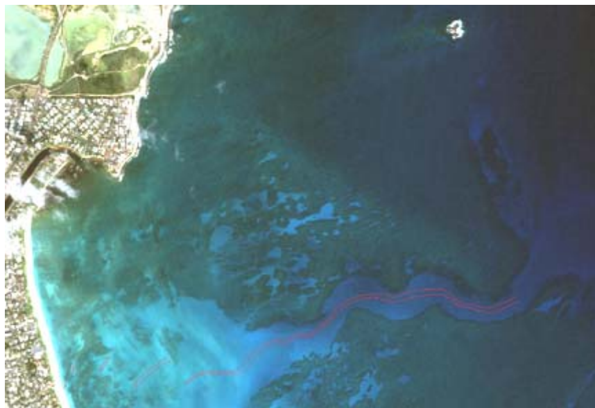
Figure 1 Kailua Bay, Hawaii. This is an orthorectified Quickbird Satellite image with 2.4m pixel resolution. Blue, Green, and Red bands are used for image analysis. The red lines are pixels selected to compute a data rotation with a depth band.
