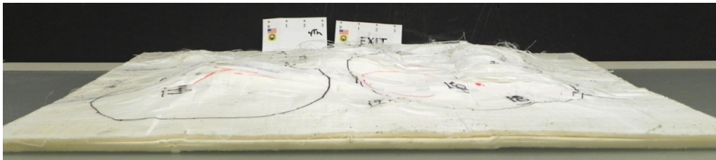
Figure 7. Side 2 edge shear on panel 3.
