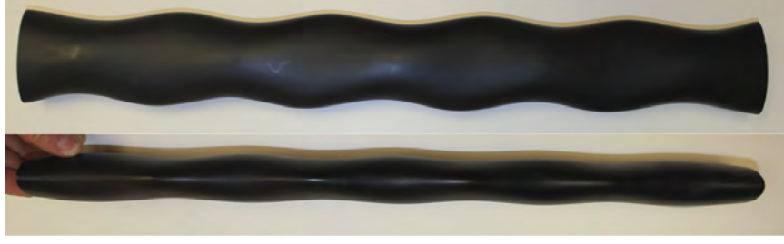
Figure 2-2: (Top) Side view and (Bottom) front view of a fabricated replica of the whisker test section, capturing the asymmetric undulatory geometry. Stereolithography was used to create this plastic hollow structure. Dimensions were taken directly from [58] and enlarged by a factor of 50.
