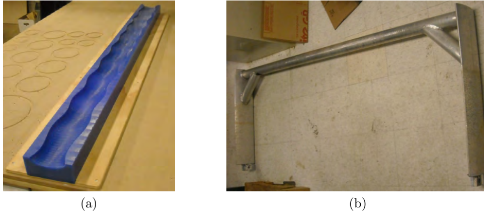
Figure C-1: (a) One half of the whisker mold, which was made from six blocks of machinable wax bolted together. A CNC tool path for the whisker geometry was created in MasterCAM from Solidworks and then routed out. (b) The mount to which the whisker was attached. The model was strung in the empty space pictured at the bottom. The two struts have an airfoil profile to minimize drag. The tube on top attaches directly to the front of the Tow Tank carriage.
