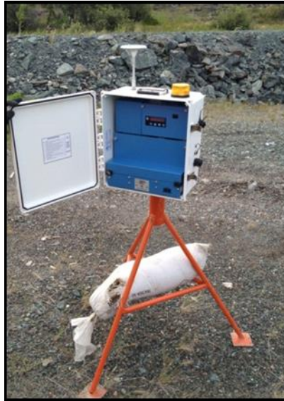
Figure C-3. ThermoScientific ADR 1500 Area Dust Monitor field deployment.
