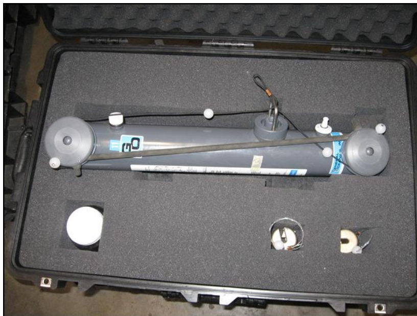
Figure C-17. GO-FLO sample bottle (USCG Gulf Strike Team package).
