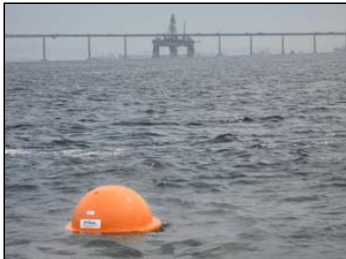
Figure C-10. MetOcean iSphere Tracking Buoy deployed.
