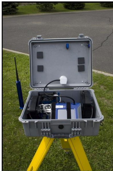
Figure C-5. TSI DustTrak DRX 8533 air monitor field deployment.
