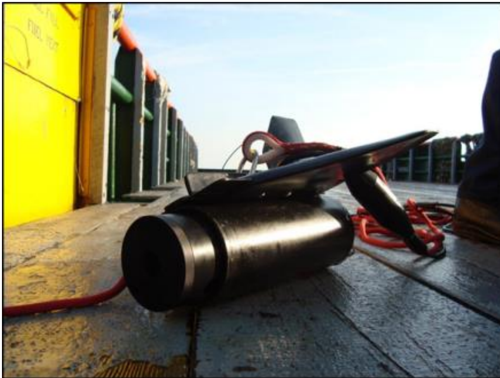
Figure A-1. Turner Designs C3™ fluorometer in specially constructed housing.
