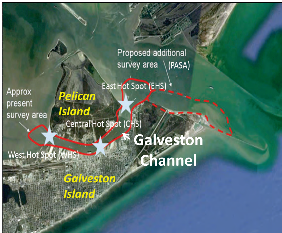
Figure 10. February–March 2010 field study showing three shoaling hotspots in Galveston Channel (modified from URS 2010).
