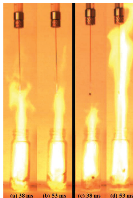
Fig. 3 [MAT][DCA] neat (a and b) and loaded with 0.33 % B milled in [MAT][DCA] (c and d) with 98 % WFNA: (a and c) first sign of ignition and (b and d) burn ongoing. The resolution was lowered to fit the larger flames: vial sizes in all runs are identical.
