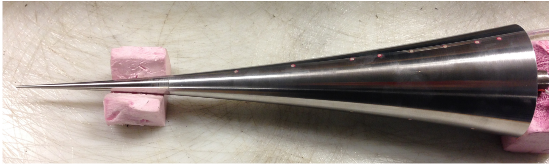
Figure 8.3. Picture of the flared cone model with blunt nose tip, showing fast pressure transducers mounted in the main ( 0^\circ ) ray.
