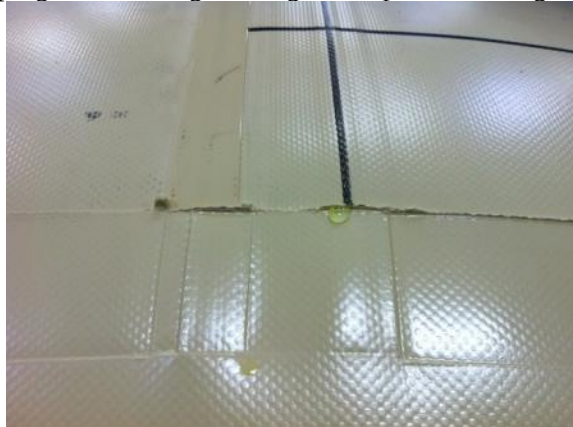
Figure 6.2.110 – Minor weeping at frame edge through un-taped scrim edge
