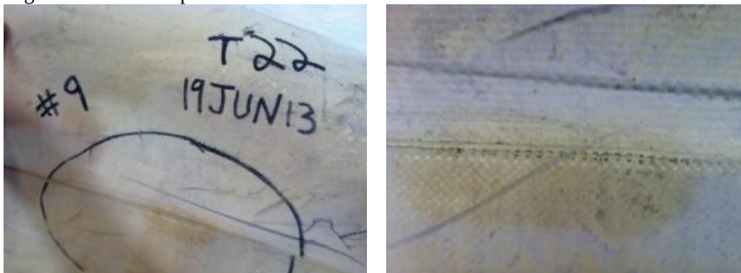
Figure 5.4.115 – No Leak Observed – T24 – Found during extraction Major wrinkle in bottom of Tank 24 closing cross seam – no leak noted, however, impossible to see in field
