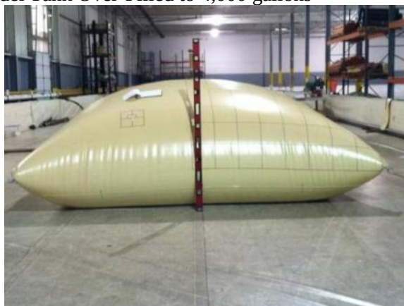
Figure 4.5.22 – FY2008 Model Tank Over-Filled to 4,000 gallons
