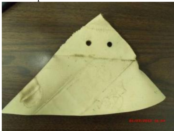
Figure 4.5.14 – Typical Welded Unclamped Corner with Clamp Holes
