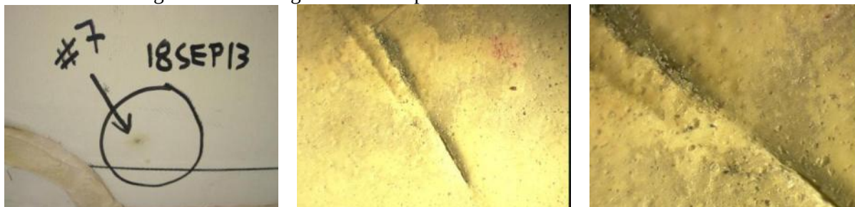
Figure 5.4.85 – Class I – T15-10 – Panel CL1 – 5 JUL 13 External surface contamination or chemical cleaning agent
