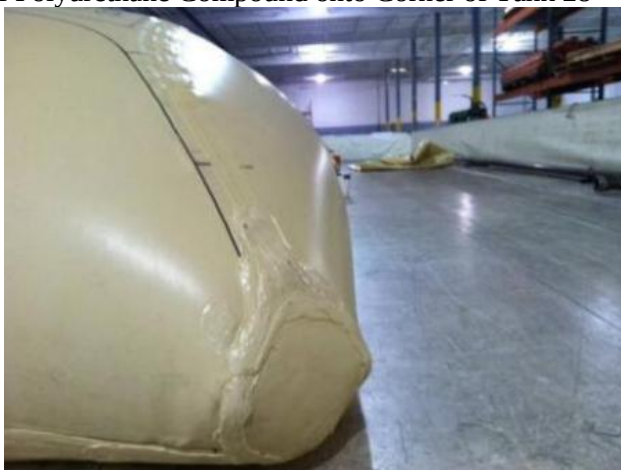
Figure 4.5.8 – Extrusion of Polyurethane Compound onto Corner of Tank 28
