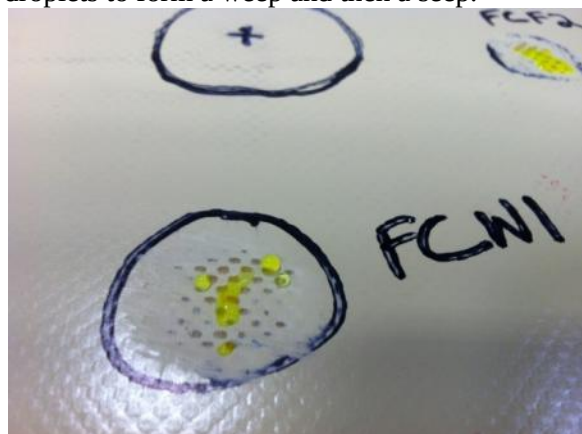
Figure 6.2.61 – View of FCW1 classic droplet formation. As droplets form out of individual fiber bundles, they combine with neighboring droplets to form a weep and then a seep.
