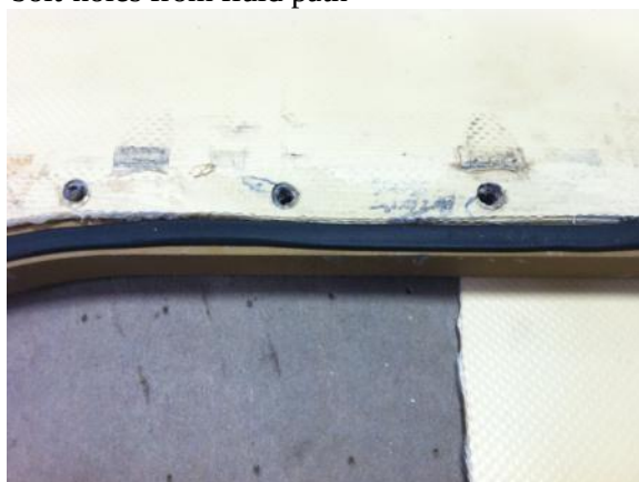
Figure 6.2.100 – Close up of additional 50 durometer O-ring isolating peripheral scrim and bolt-holes from fluid path
