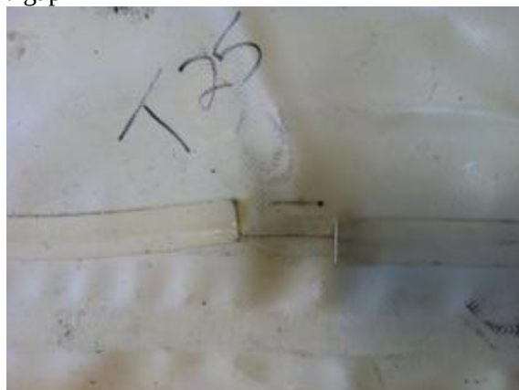
Figure 5.4.118 – T25 – No Leak – Found during extraction Internal tape overstretch tear / gap
