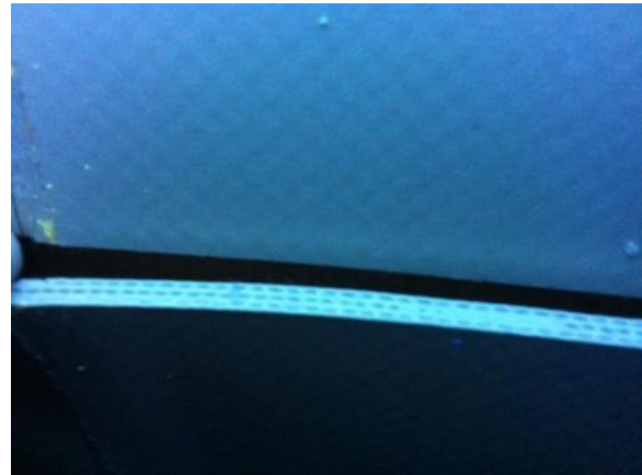
Figure 6.2.44 – Double Butt Seam cross section – minimal dye penetration internal strap, none apparent on center panels or exterior strap
