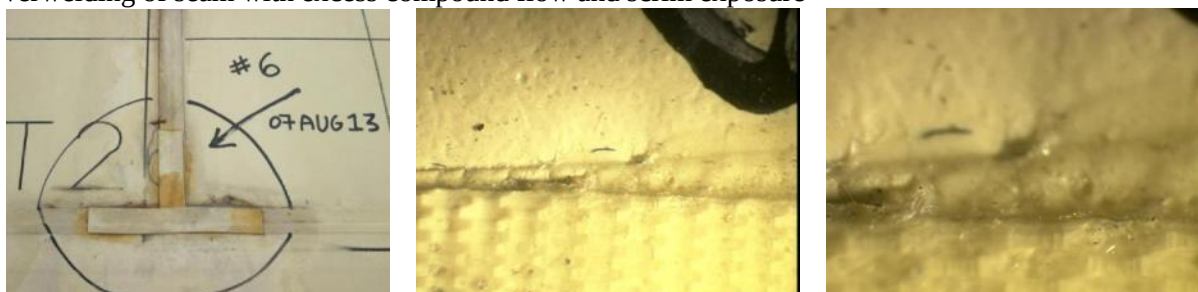
Figure 5.4.98 – Class I – T26-6 – T-Seam Closing – 7 AUG 13 Overwelding of seam with excess compound flow and scrim exposure
