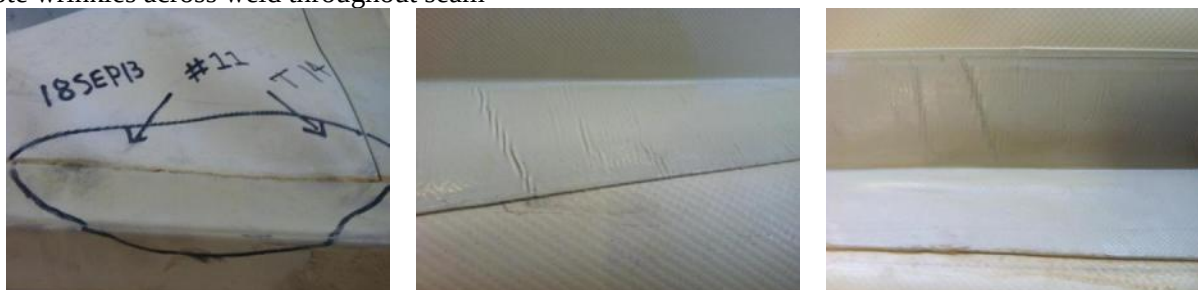
Figure 5.4.105 – Class I – T14-11 – Closing Seam – 18 SEP 13 Note wrinkles across weld throughout seam
