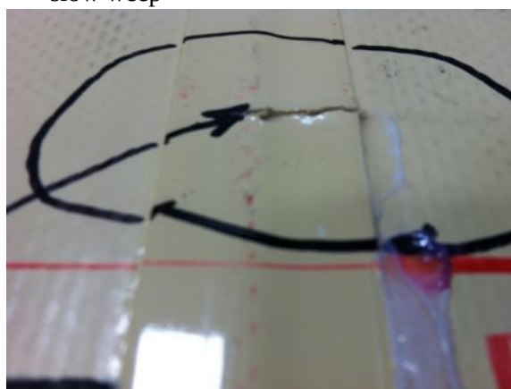
Figure 6.2.109 – External tape cut above center panel showing milky colored deposit from very slow weep
