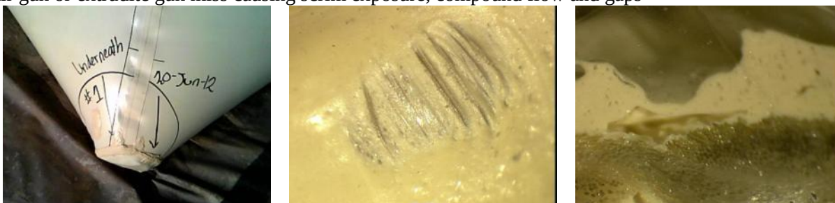
Figure 5.4.82 – Class II – T28-1 – Corner – 20 JUN 12 Air gun or extrudite gun miss causing scrim exposure, compound flow and gaps
