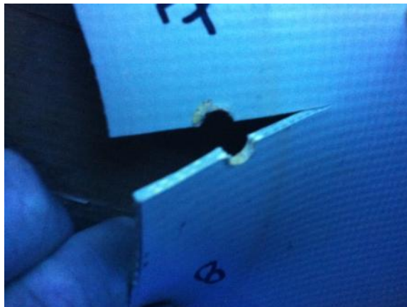
Figure 6.2.96 – Dye penetration in material scrim for bolt-hole 7
