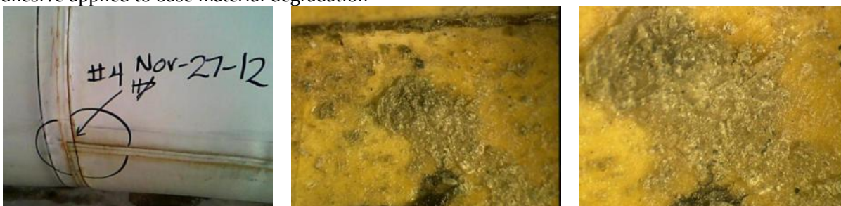
Figure 5.4.81 – Class II – T24-4 – T-Seam Closing – 27 NOV 12 Adhesive applied to base material degradation
