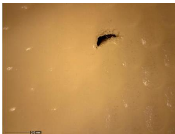
Figure 6.2.70 – At pressure of 15 in H 2 O, leak became profuse
