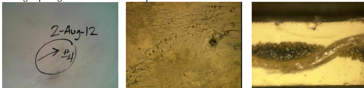
Figure 5.4.88 – Class I – T18-4 – Panel – 2 AUG 12 Hot air gun pitting or abrasion with subsequent contamination
