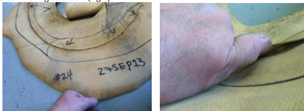
Figure 5.4.108 – Class I – T17-24 – Vent Doubler – 27 SEP 13 Vent reinforcement ring cold weld (right)
