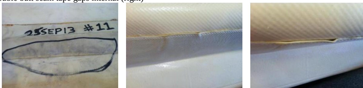
Figure 5.4.106 – Class I – T15-11 – Closing Seam Tape – 25 SEP 13 Double butt seam tape gaps internal (right)
