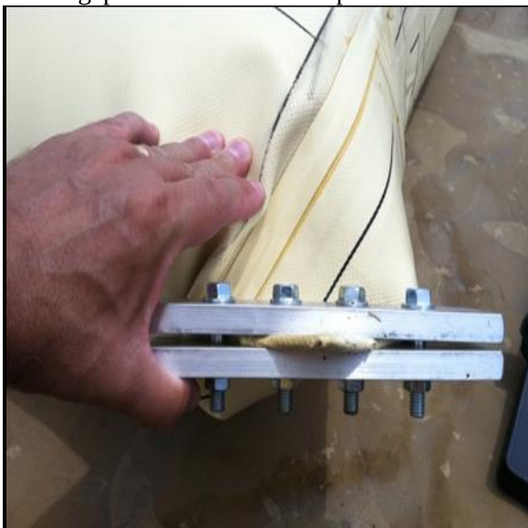
Figure 4.5.16 – Clamp Plates Cantilevered – narrower gap on outside between plates
