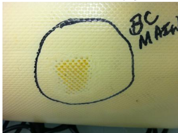
Figure 6.2.57 – Internal backside abrasion – extensive dye penetration
