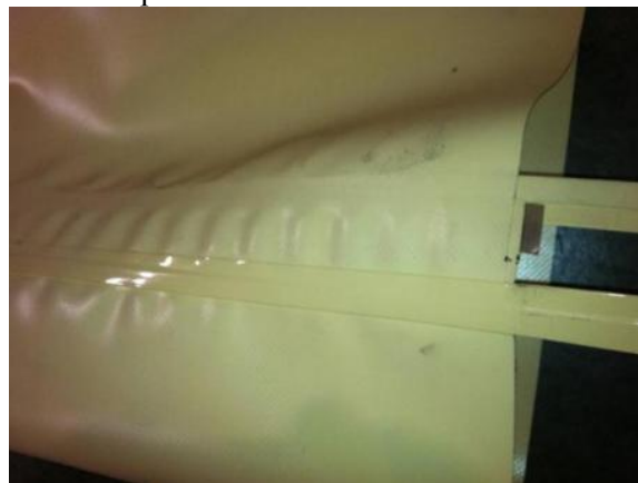
Figure 4.5.2 – Top Blanket Weld Showing Profile Tape “Pucker”
