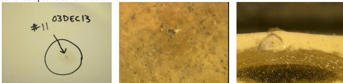
Figure 5.4.99 – Class I – T26-11 – Panel – 3 DEC 13 Internal compound contamination
