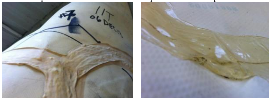
Figure 5.4.102 – Class I – T11-7 – Corner – 6 DEC 13 Exposed scrim on corner patch under clear extrudite compound on internal panel
