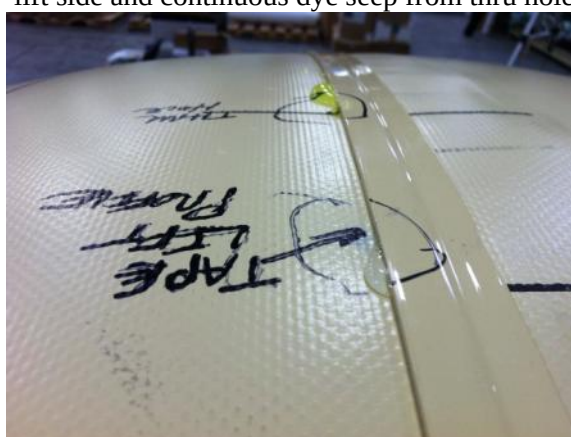
Figure 6.2.119 – Clear weep from profile tape lift side and continuous dye seep from thru hole
