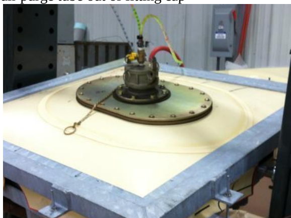
Figure 6.2.90 – Tank fitting showing additional air purge tube out of fitting cap
