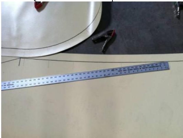
Figure 4.5.7 – Complex Radius on Quonset Hut which Requires Additional Match Marks
