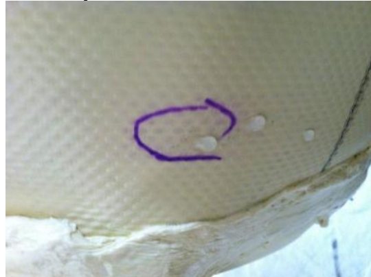
Figure 4.5.24 – Flaw in Panel Created by Internal Hot Air Gun Miss at Corner
