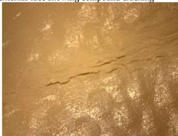
Figure 6.2.80 – Weep produced at beginning of second day of testing, right after reaching pressure
