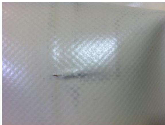
Figure 6.2.108 – Backside of tape lift indicating of breach in compound (on left)
