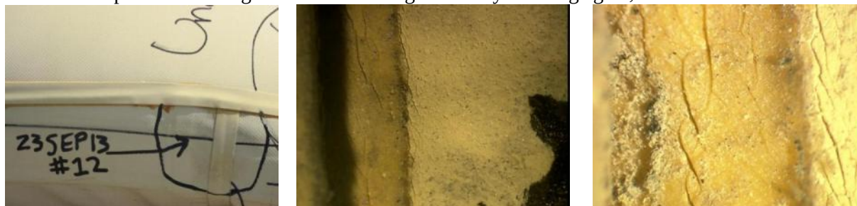
Figure 5.4.90 – Class I – T20-12 – T-Seam Closing – 23 SEP 13 Localized compound stiffening and stress cracking caused by cleaning agent, adhesive or both
