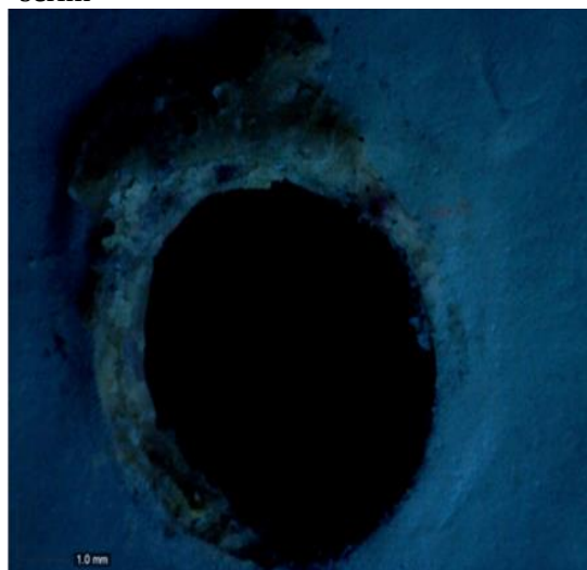
Figure 6.2.104 – Close up black light of bolt-hole 15 with no apparent dye penetration in scrim
