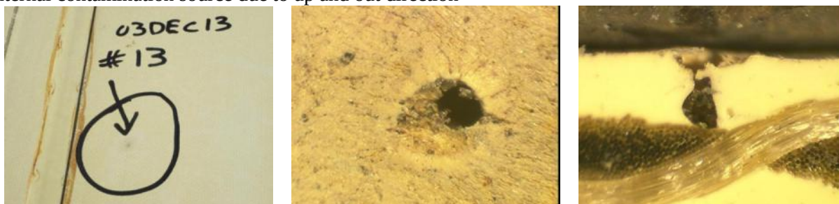
Figure 5.4.94 – Class I – T24-13 – Panel – 3 DEC 13 Internal contamination source due to up and out direction
