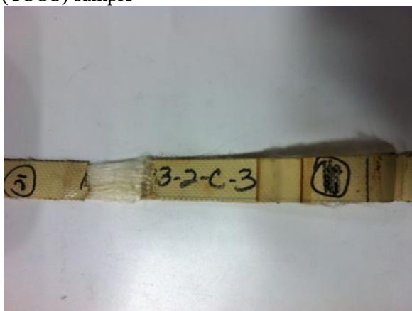
Figure 6.1.12 – Yarns Stripped out of Seam (YSOS) sample
