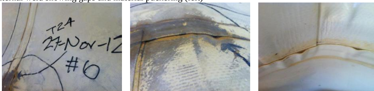
Figure 5.4.116 – Class I – T24-6 – T-Seam Closing – 27 NOV 12 Internal weld showing gaps and material puckering (left)
