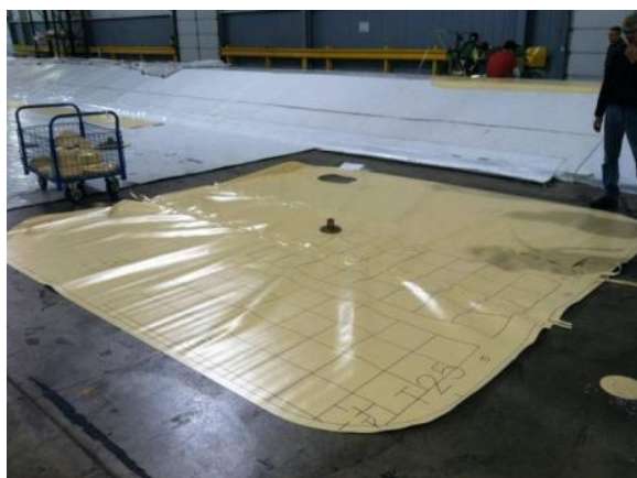
Figure 4.5.1 – Belly Band (Tank 25) Top Blanket Welded
