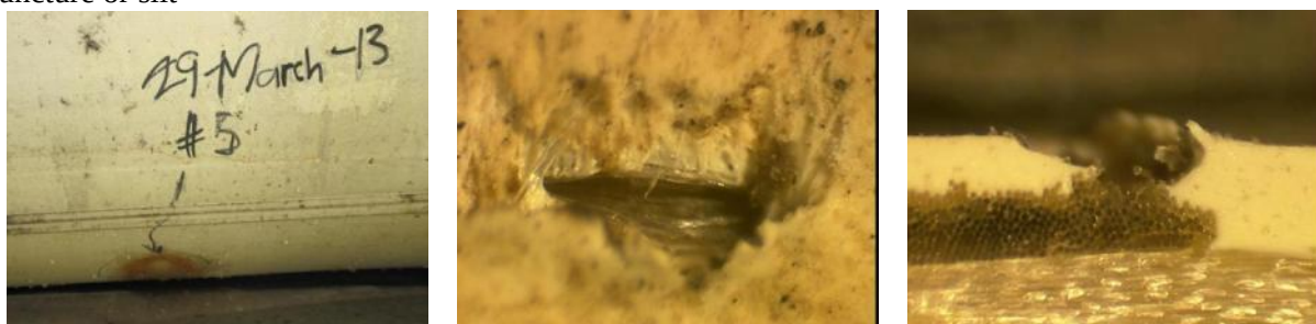
Figure 5.4.97 – Class I – T26-5 – Panel – 29 MAR 13 Puncture or slit
