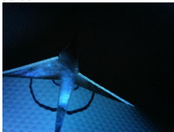
Figure 6.2.123 – Cross-sectional cut of 0.013 pin hole – dye penetration reduces the further from the hole
