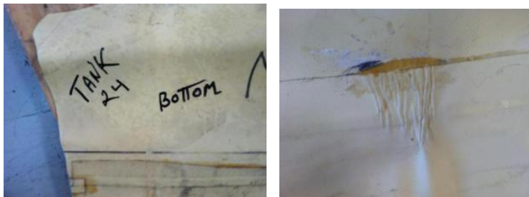
Figure 5.4.115 – No Leak Observed – T24 – Found during extraction Major wrinkle in bottom of Tank 24 closing cross seam – no leak noted, however, impossible to see in field
