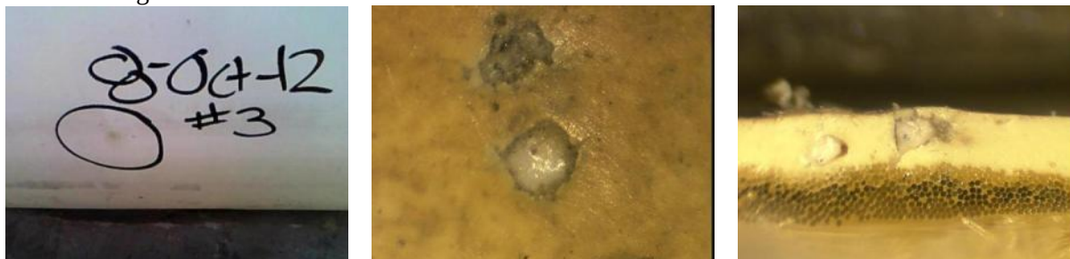
Figure 5.4.92 – Class I – T24-3 – Panel – 8 OCT 12 Internal coating contamination
