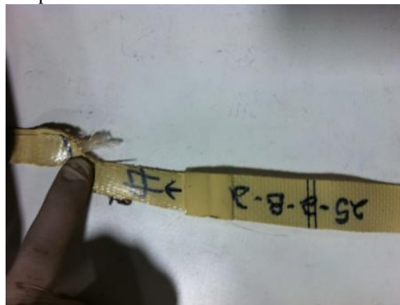
Figure 6.1.11 – Torn Outside of Weld (TOW) sample
