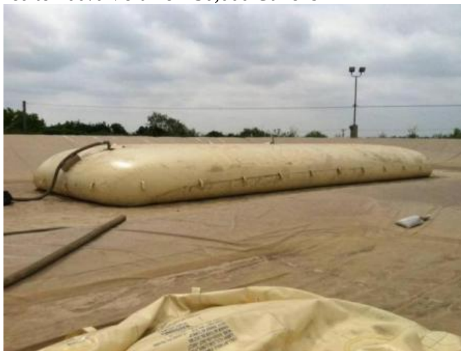
Figure 5.3.3 Tank Filled to 100% Volume – 50,000 Gallons
