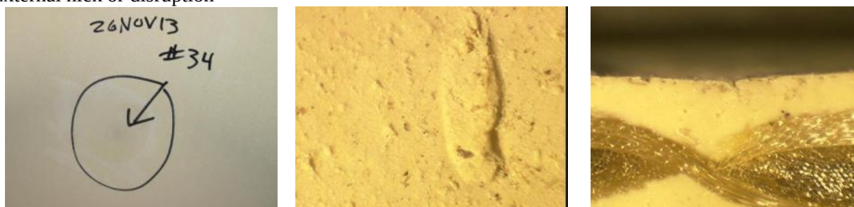
Figure 5.4.89 – T19-34 – Class I – Panel – 26 NOV 13 External nick or disruption
