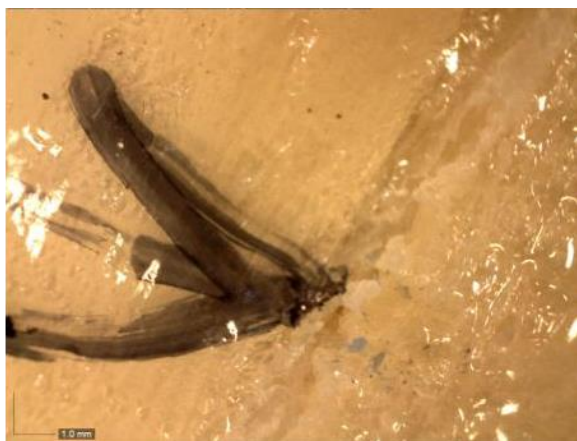
Figure 6.2.111 – Internal tape lift through heavy adhesive compound
