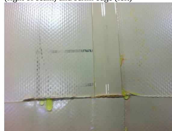
Figure 6.2.121 – Residual flow form thru hole (right of seam) and scrim edge (left)
