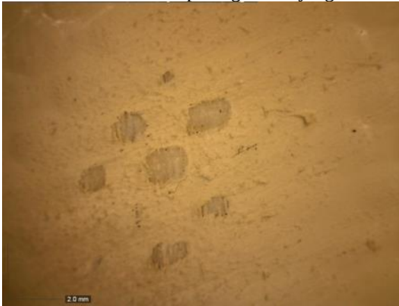
Figure 6.2.47 – Internal surface compound removed with abrasive wheel exposing underlying scrim
