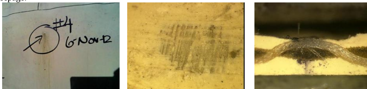
Figure 5.4.95 – Class I – T25-4 – Panel – 6 NOV 12 Abrasion with fibers coming to surface only. No fiber bundle disruption hence did not manifest Class II seepage.
