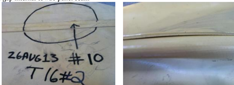
Figure 5.4.108 – Class I – T17-24 – Vent Doubler – 27 SEP 13 Vent reinforcement ring cold weld (right)
