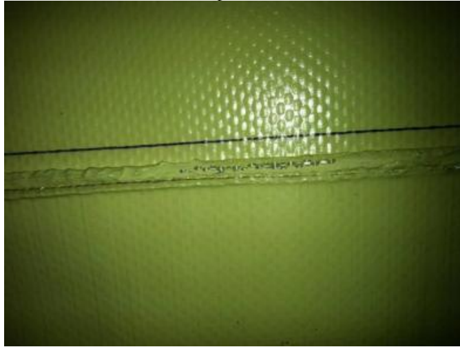
Figure 4.5.18 – Exposed Fiber Bundle Due to Compound Overflow
