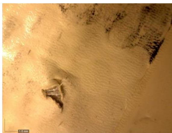
Figure 6.2.112 – Resultant external compound breach
