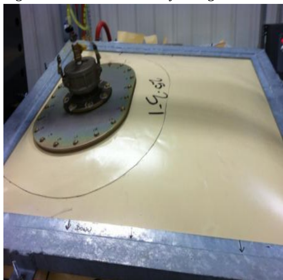
Figure 6.2.97 – Tank manway fitting
