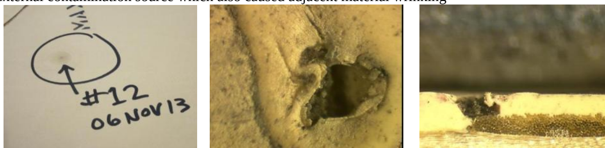
Figure 5.4.93 – Class I – T24-12 – Panel – 6 NOV 13 External contamination source which also caused adjacent material wrinkling
