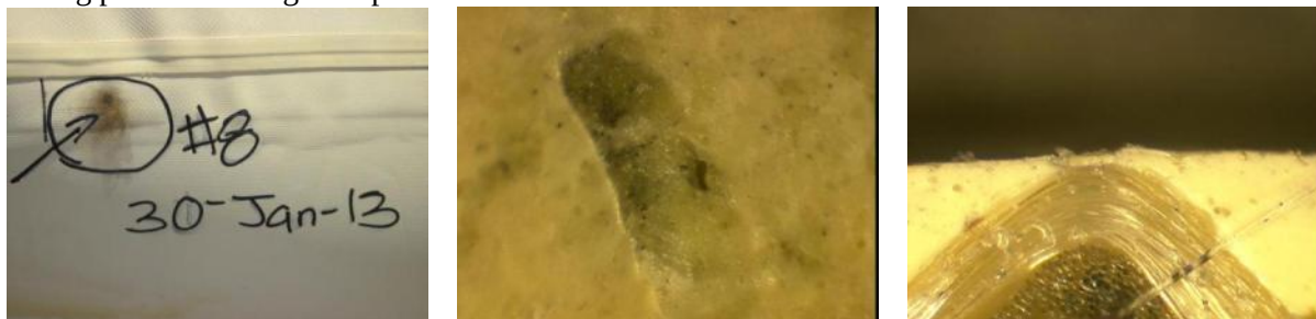
Figure 5.4.96 – Class I – T25-8 – Closing Seam – 10 JUL 13 Welding process coating disruption
