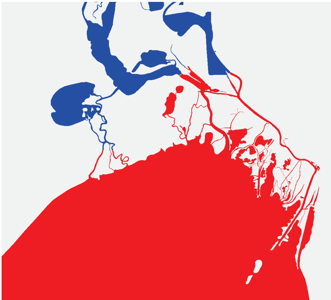
Figure 8-7 Initial salinities for wet-season salinity simulation. Red is 30 psu and blue is 0 psu.
