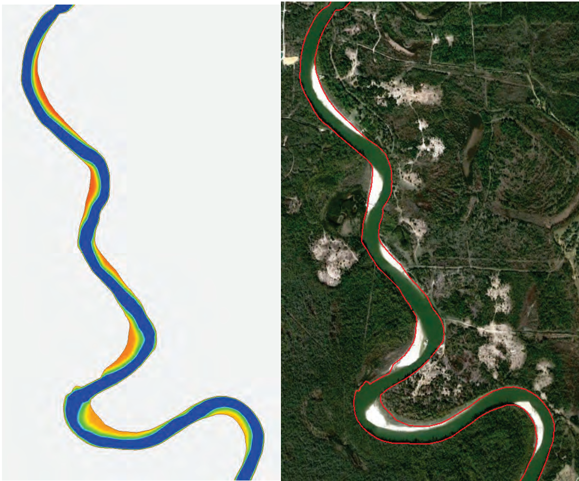
Figure 6-3 Example of the estimation of point bars along the upper meandering Trinity River. Red indicates shallow areas; blue indicates deep areas. See Appendix B for details.
