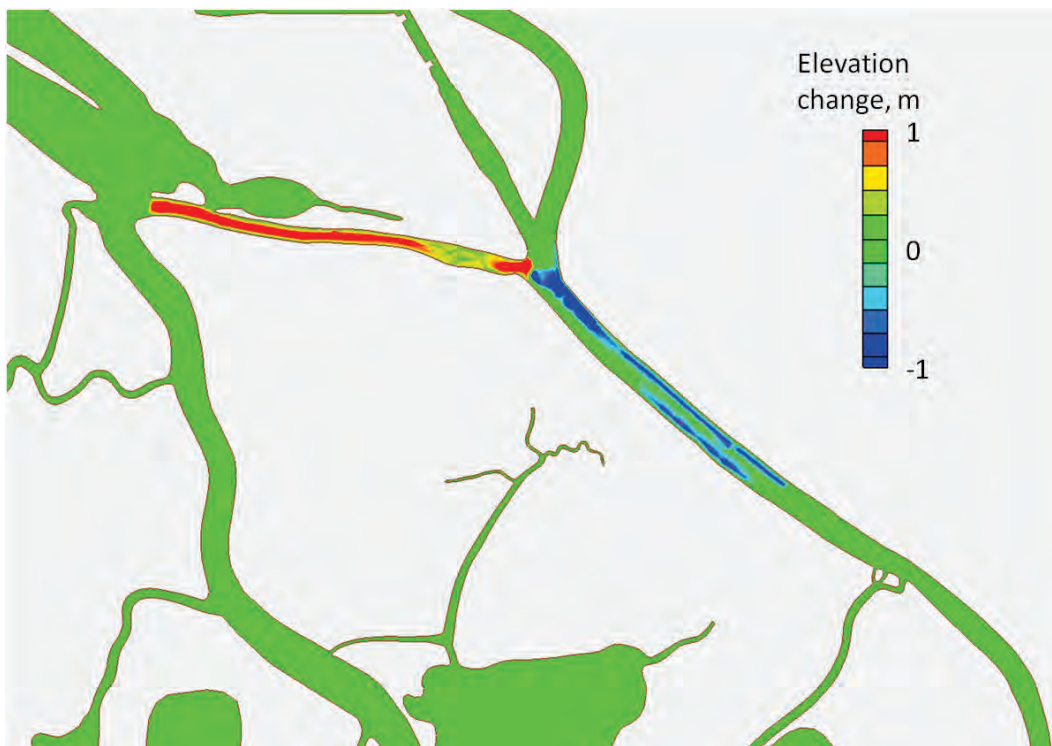
Figure 8-2 Bed changes as a result of dredging Trinity River shoal and placing the material in ORCO.
