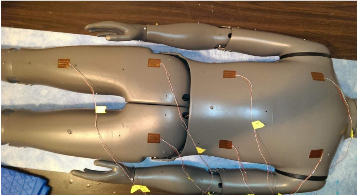
Figure 62. Example placement of heat flux sensors on a thermal manikin
