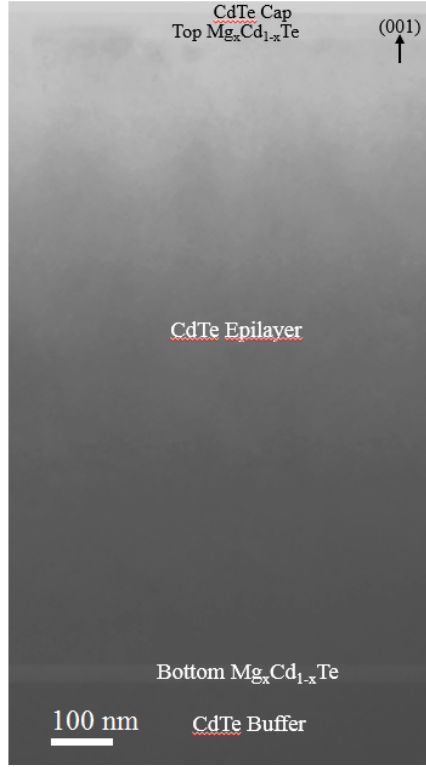
Fig. 2. Bright-field TEM image showing the high structural quality of a CdTe/MgCdTe DH grown at 265°C.
