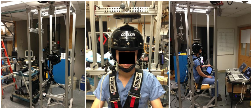
Figure 8 Solenoid powered traction system for applying cyclic loads in-vivo
