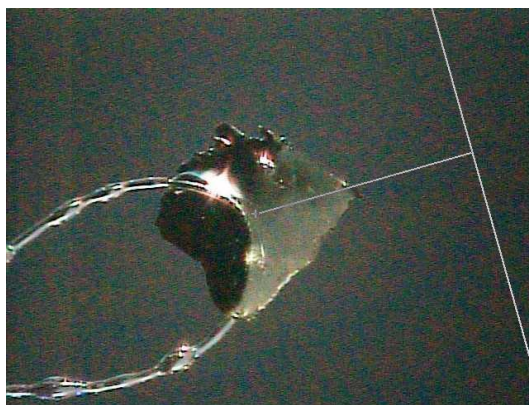
Figure D.20 Photograph of single crystal of Co-BTTB-DMBPY (size (mm) – 0.128 x 0.536 x 0.555).
