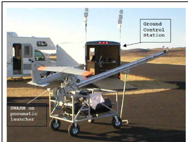
Figure 2. GCS for Smart Warfighting Array of Reconfigurable Modules (SWARM) program UAS from Naval Surface Warfare Center, Carderock Division (NSWCCD) at McMillan Airfield, Camp Roberts, CA NG Base (Source: Figure 3, Butner thesis (2002) p. 19.)
