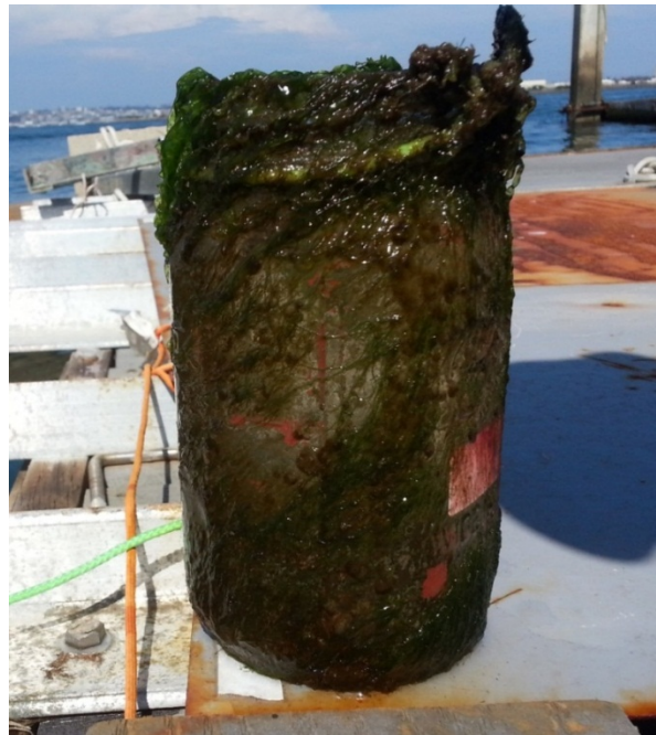
Figure 22. Jar with anti-foul coating (no heating) after 45 days.
