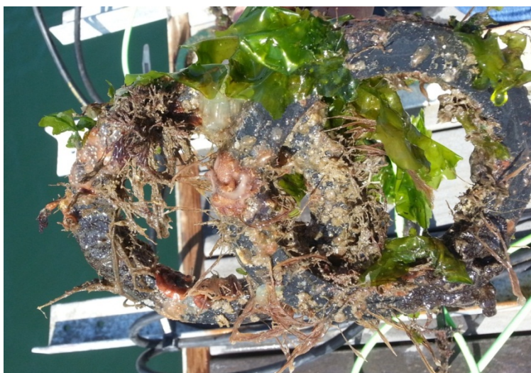
Figure 16. Top view of rings (no anti-foul) after 45 days.
