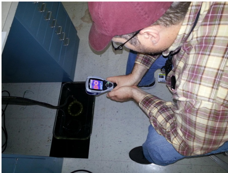
Figure 4. Thermal imaging using FLIR® camera.
