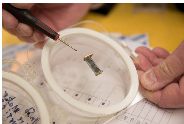
A lopsided tuning fork, made of the semiconductor indium antimonide, used in the experiment. Kevin Fitzsimons, The Ohio State University, CC BY-NC-ND
