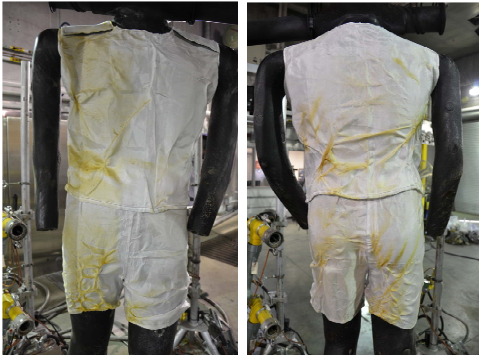
Figure 36. Manikin test of UHMWPE 375D woven fabric under Defender M coveralls on Day 2.
