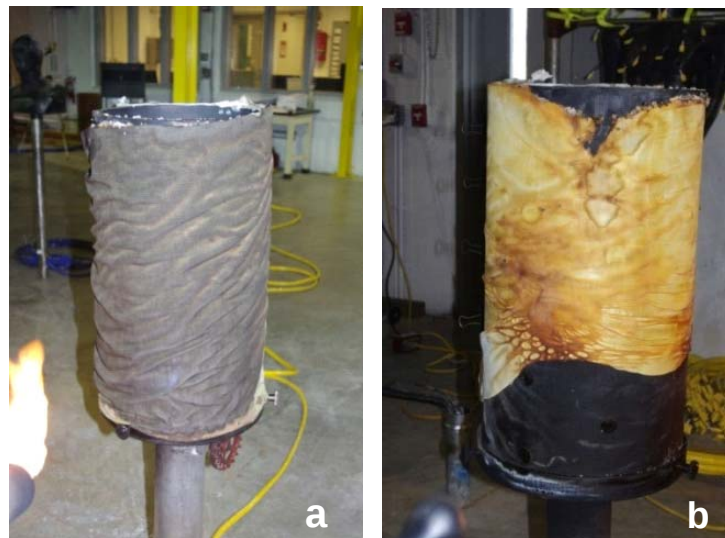
Figure 16. Cylindrical midscale test of Defender M and UHMWPE 375D plain weave after test: a) Outer layer; b) Under layer.
