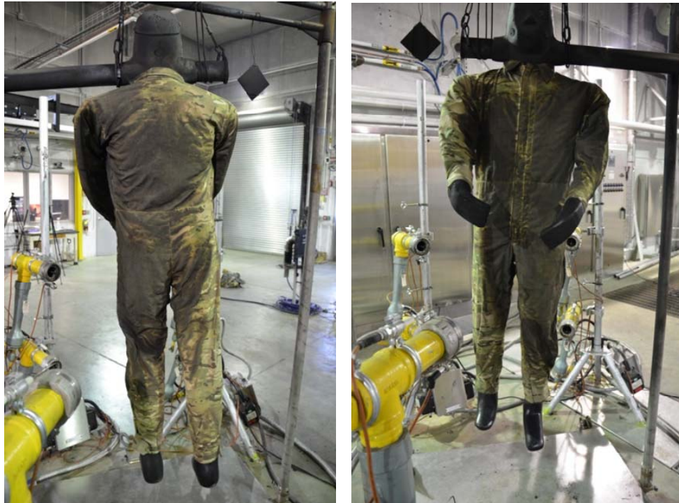
Figure 29. Manikin Test of Defender M coveralls tested with no undergarments.
