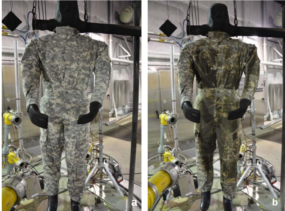
Figure 31. Manikin test of FRACU: a) Before testing; b) After testing.
