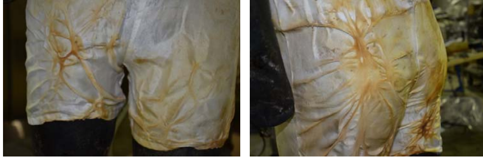
Figure 35. Close up of manikin test damage to UHMWPE 375D woven shorts.
