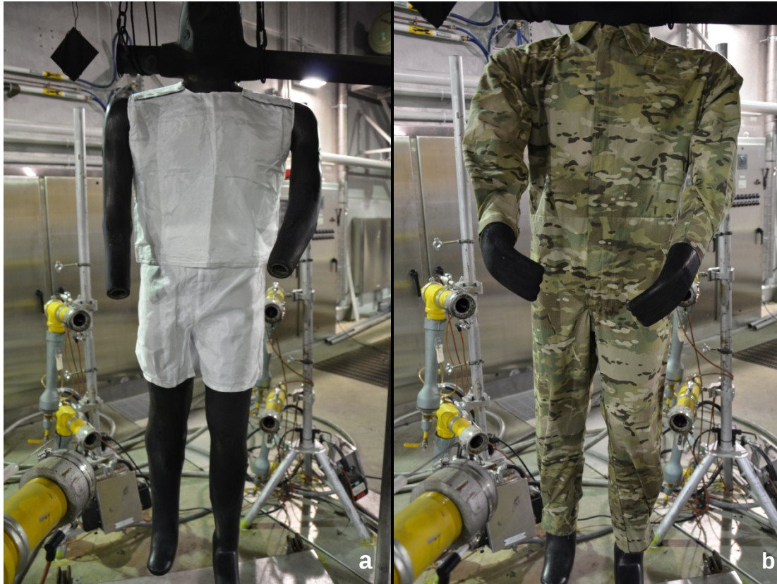
Figure 9. Test garments on thermal test manikin: a) Vest and boxer shorts; b) Defender M coverall.
