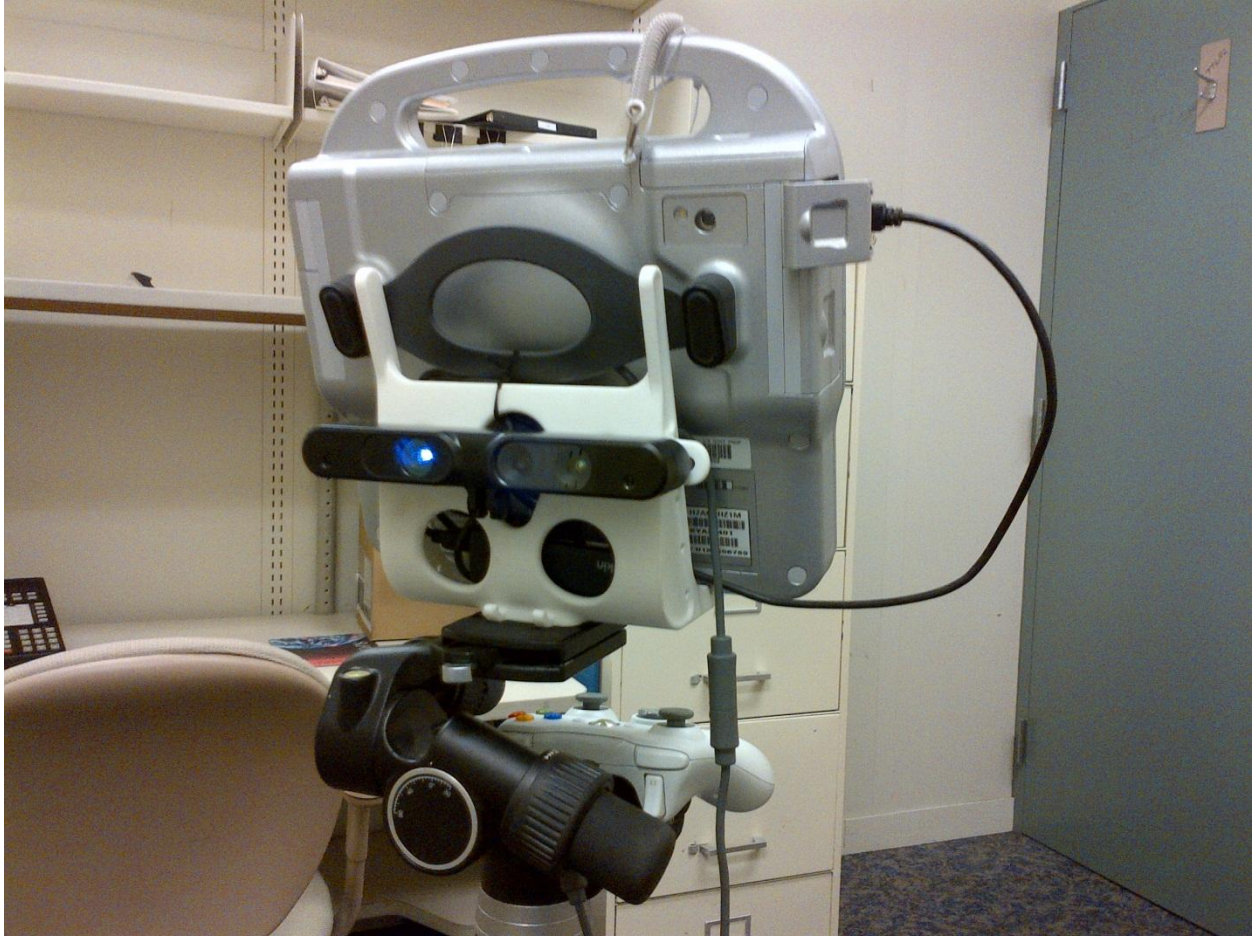
Figure 3-27. The ASUS sensor attached to the custom bracket
