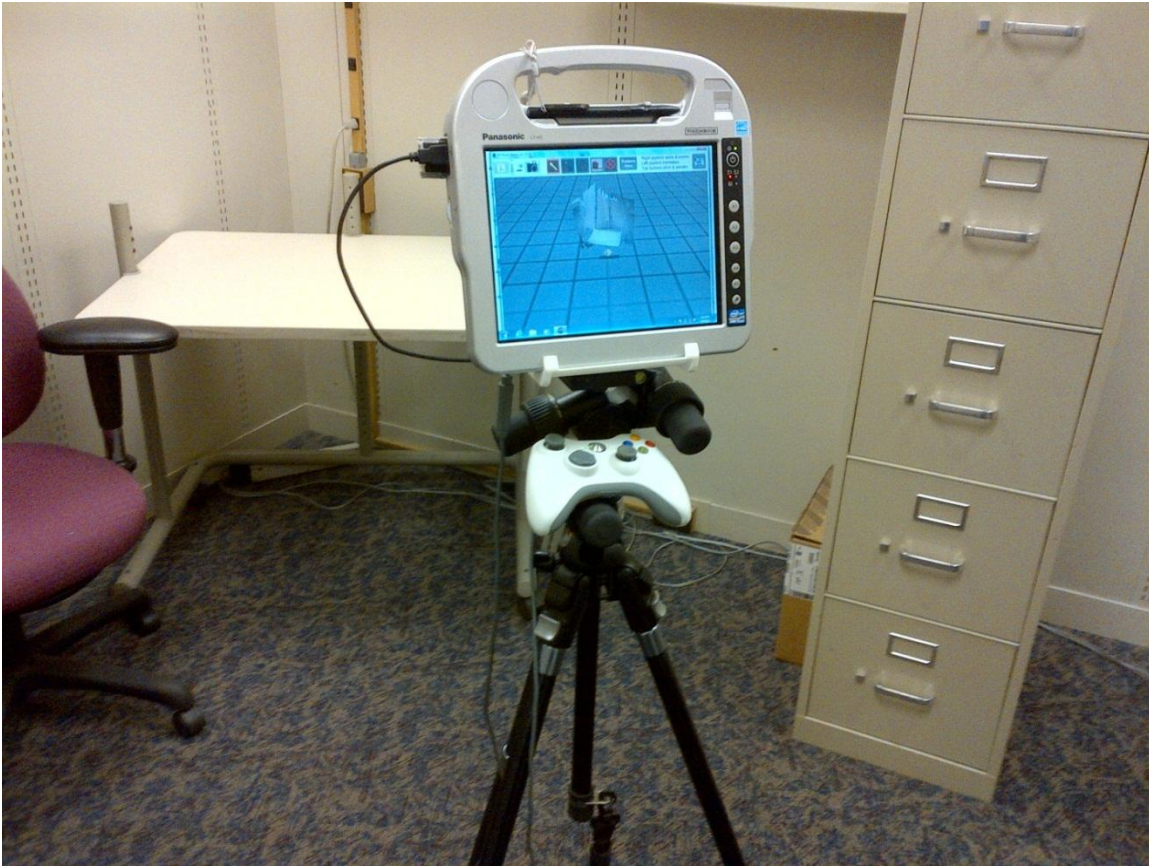
Figure 2.6 – 3D sensor and tablet configuration for SESSA
