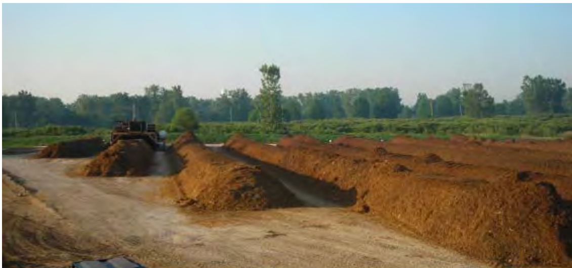
Figure 57. Windrow composting requires a large area.
