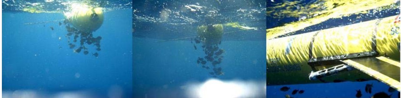
Fig. 5. The fish schooling under the Webb glider at the end of the RIMPAC deployment. The fish are observed to be schooling directly under the glider by the optical sensors. The CTD upon close inspection is bent by almost 30 degrees suggesting blunt upward trauma from below.
