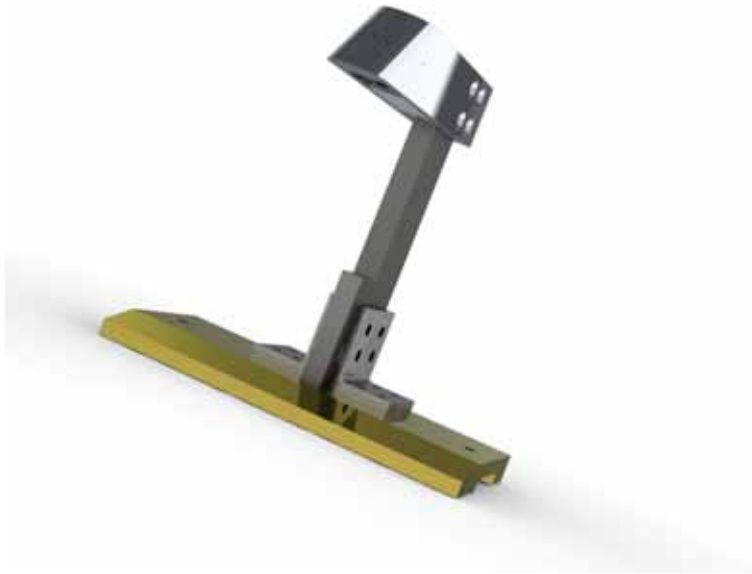
Figure 3.12: Rendering of the 45° aluminium swept-cylinder fin to be used for pressure/temperature sensitive paint measurements and piezo-electric pressure sensing.
