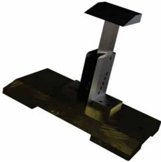
Figure 3.15: Rendering of the aluminium shock generator to be used in all experiments where Edney Type IV interactions are desired.
