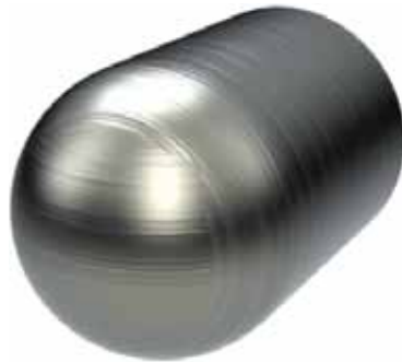
Figure 3.13: Rendering of the 45° Macor swept-cylinder fin to be used for infrared thermography.
