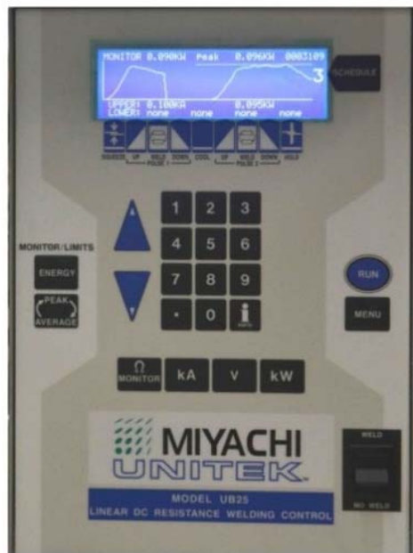
Figure 17. Front side of the Miyachi Welder. Note the waveform display screen at the top.
