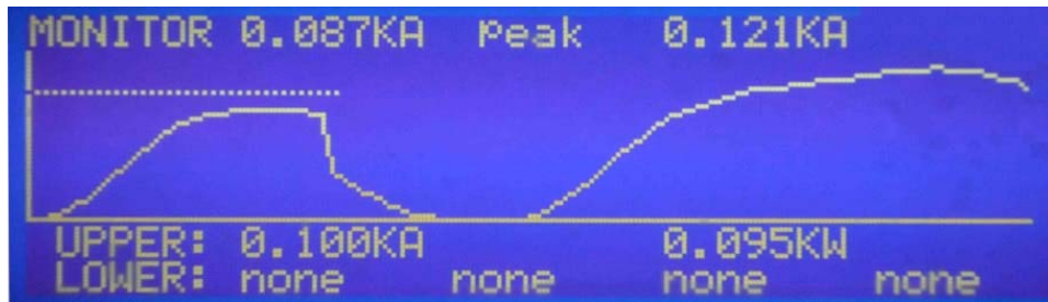
Figure 20. Welder current for a typical weld operation
