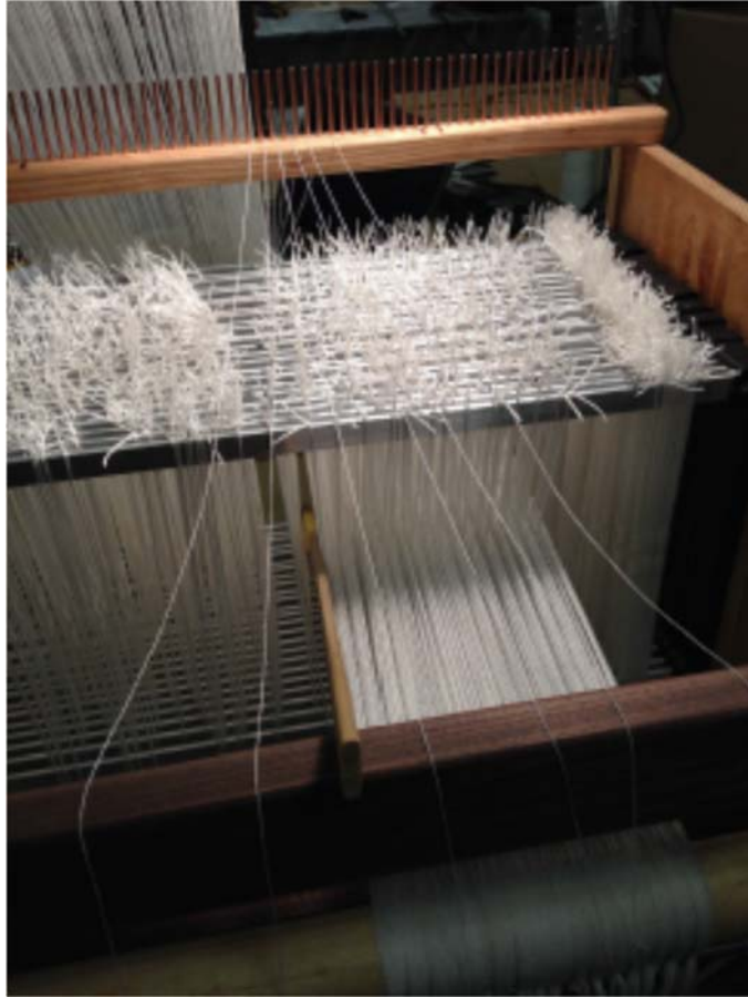
Figure 27. A group of nine warp yarns (three of which have been entered) is released from the stick to be entered into the heddles.
