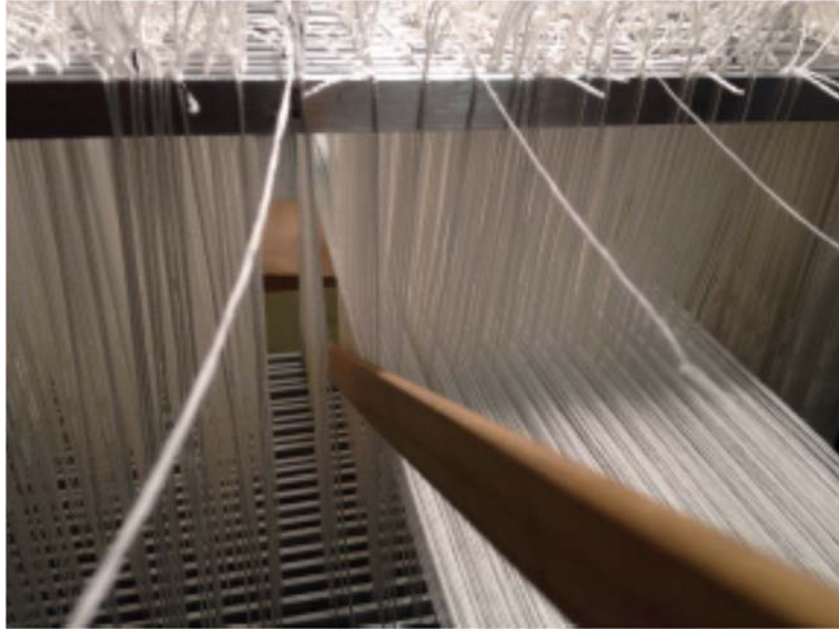
Figure 28. Heddles are separated from each other to increase the visibility of the currently engaged group and to minimize the possibility of mis-entering
