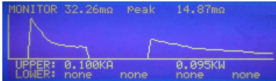
Figure 21: Interface resistance for a typical weld operation
