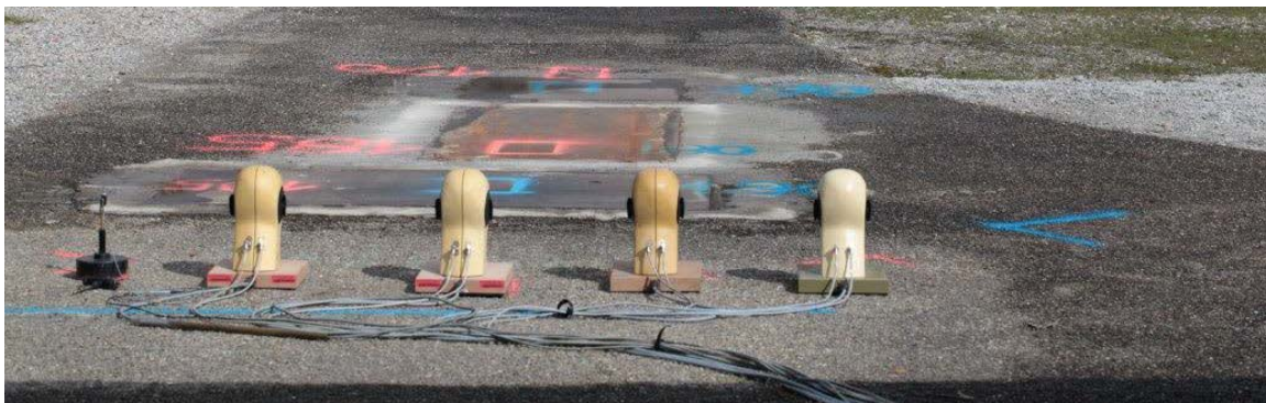
Figure 8: Placement of ATFs and free-field pressure transducer
