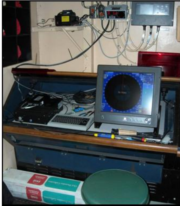
Figure 13. Rutter radar processor setup on the USCGC Healy.
