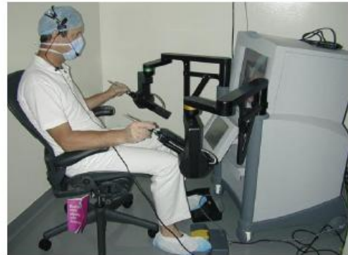
Figure 1. ZEUS Surgical Research Robot
