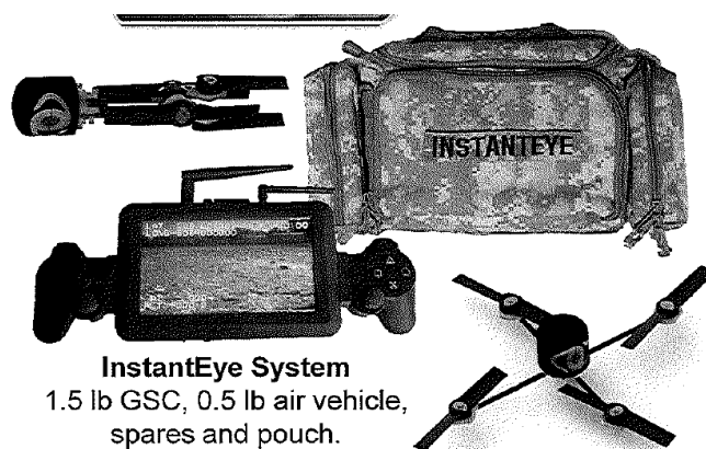
Fig. 12 InstantEye system composed of visual display and control unit, air vehicle, spares, and carrying pouch
