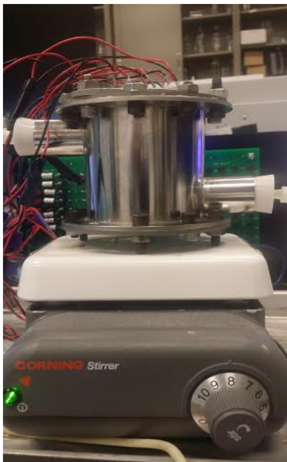
Figure 12 - Mechanically mixed UV reactor with Corning Stirrer
