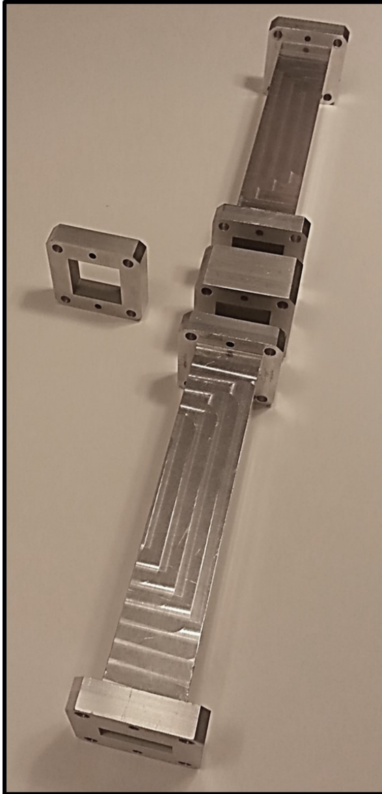
Figure 28. WRWS showing waveguide transition on either side of the sample holder, line standard is placed left of sample holder
