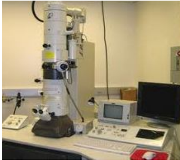
Fig. 2.11 Photograph of a typical TEM instrument.
