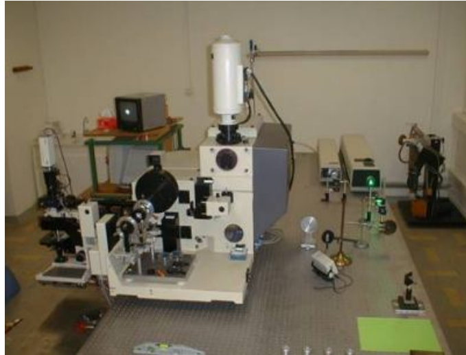
Fig. 2.12 A Jobin-Yvon T-64000 Triple-mate Raman instrument.
