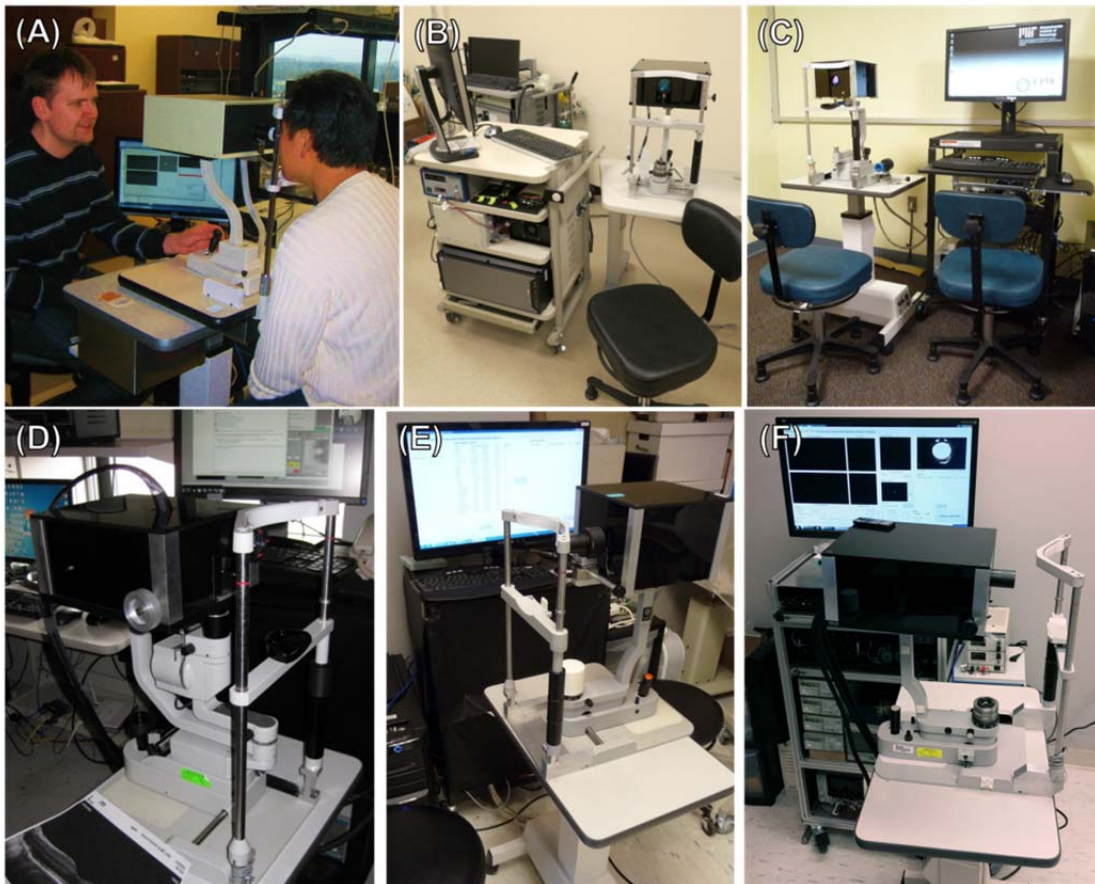
Figure 13. OCT imaging instruments were developed and deployed to the ophthalmology clinics at multiple collaborator sites. (A) 100 kHz retinal and (B) anterior imaging SS-OCT systems at OHSU. (C) 100 kHz retinal SS-OCT system at UPMC. (D) 91 kHz ultrahigh resolution retinal SD-OCT, (E) 100 kHz retinal SS-OCT, and (F) 400 kHz retinal VCSEL SS-OCT at NEEC.
