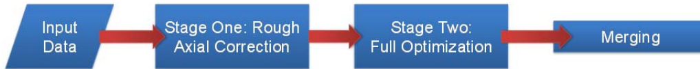
Figure 11. Improved, two stage, motion correction algorithm. The first stage performs a rough compensation of tilt using multi-resolution optimization. The tilt-corrected volumes are then used for a full optimization in stage two.
