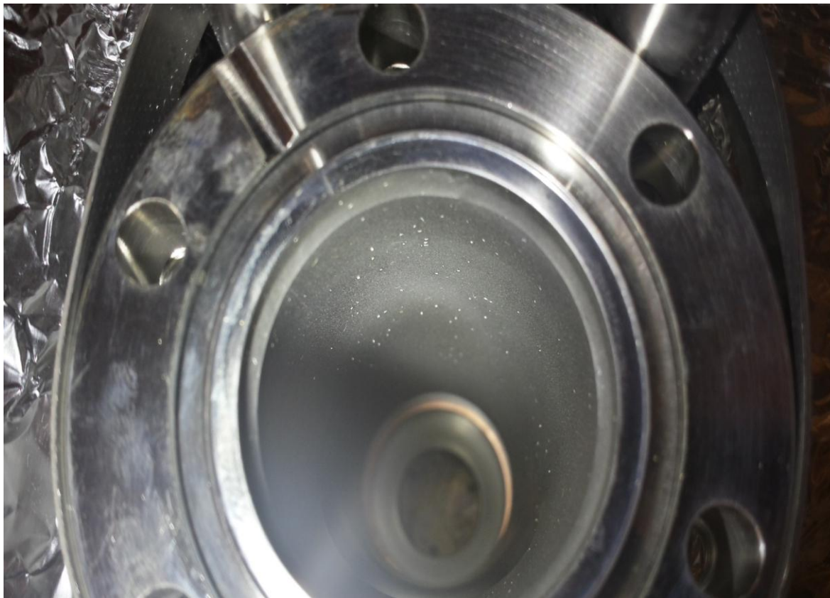
Fig. 10. The interior of the AMD chamber after the depletion of approximately 10 AMD strips over the course of several months. White specks had formed around the inside of the chamber. Due to Outgassing of the stainless-steel chamber, these were probably alkali metal hydrides, formed from rubidium vapor from the AMD and hydrogen from the stainless-steel.
