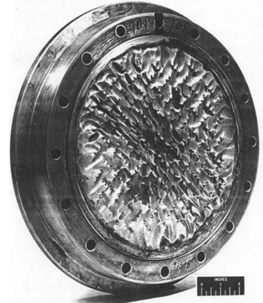
Damaged engine injector faceplate caused by combustion instabilities
