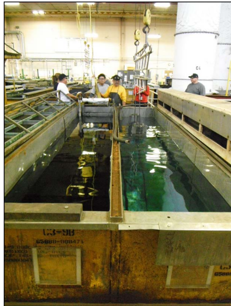
1800-gallon Surtec 650V tank (l) and rinse tank (r)
