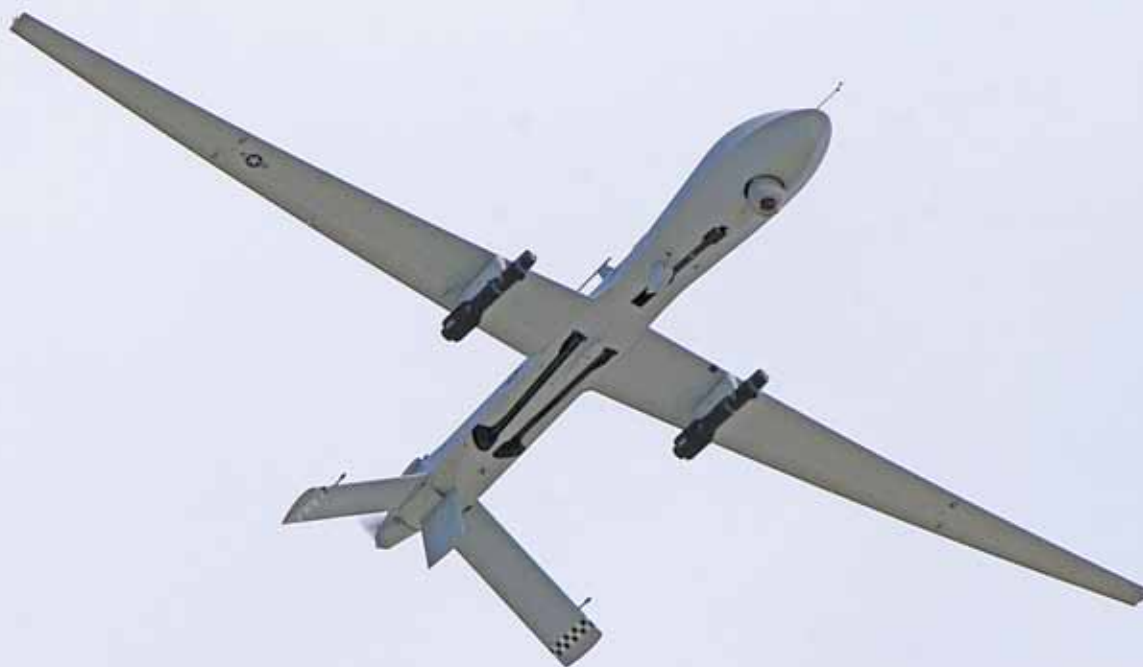
MQ-1 Predator UAV, armed with AGM-114 Hellfire missiles
