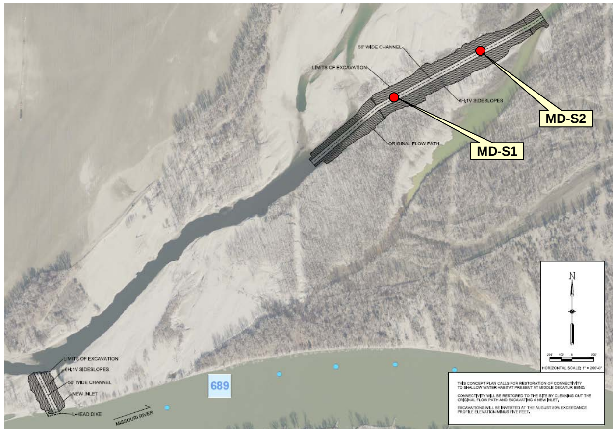
Figure 2. Proposed area to be excavated to restore shallow-water habitat at the proposed Middle Decatur project area. Locations where sediment/soil samples were collected are shown.
