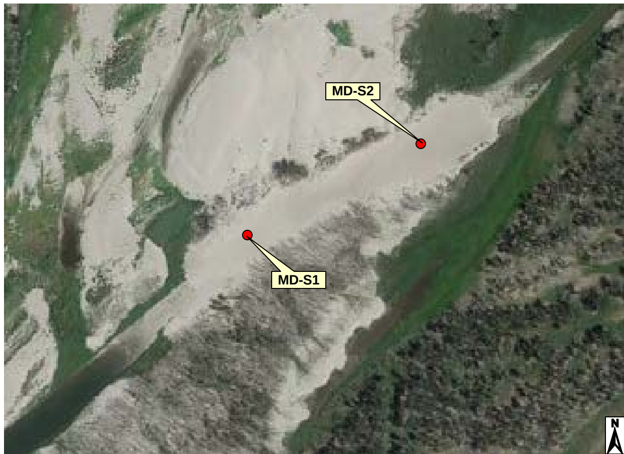
Figure 3. Locations of sites where sediment/soil samples will be collected for analysis and elutriate testing. (Site locations shown on 18-July-2012 Google Earth aerial photo of proposed project site.)
