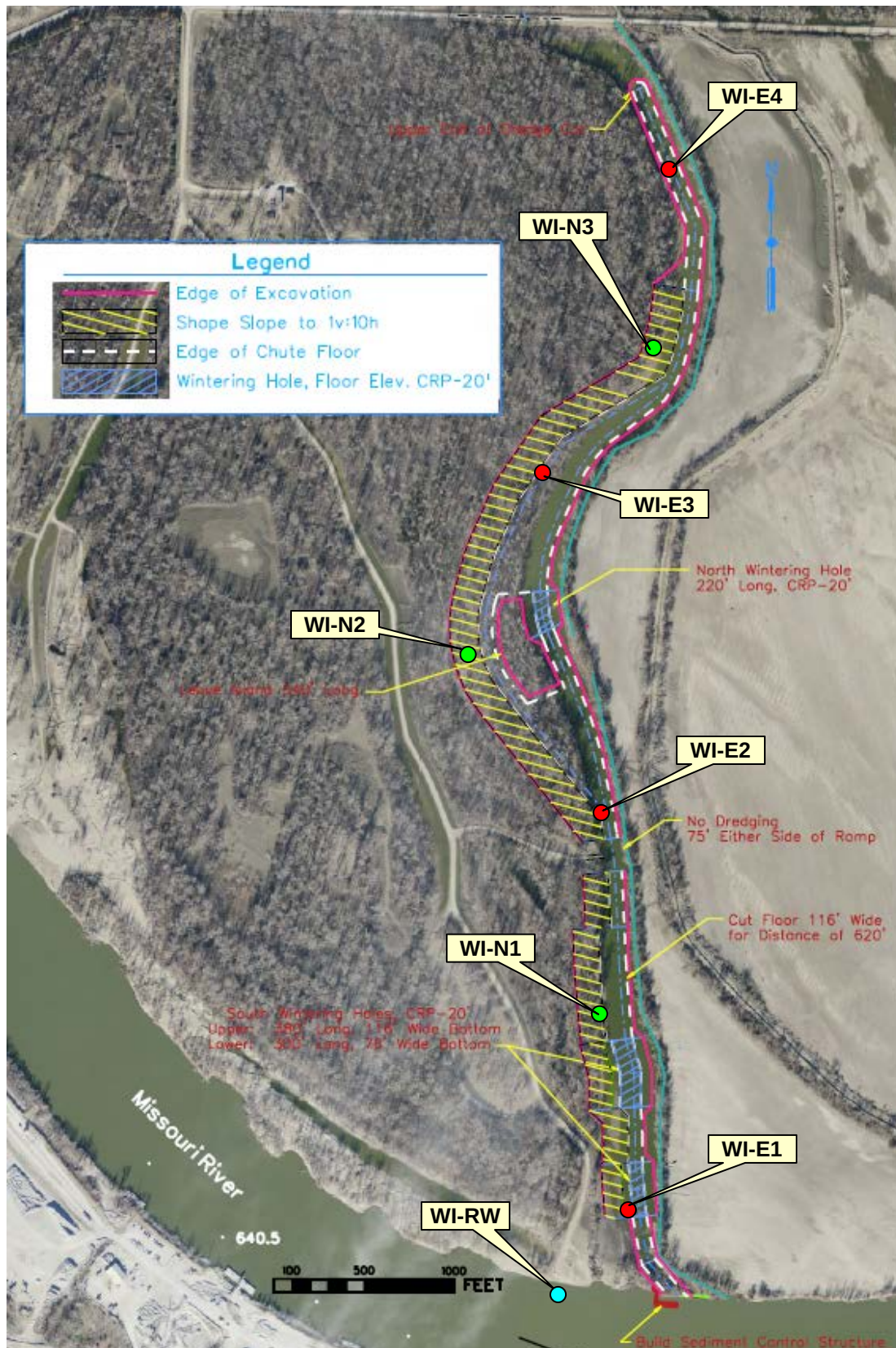
Figure 2. Proposed area for excavation to enhance and expand the existing chute at the Wilson Island project site.
