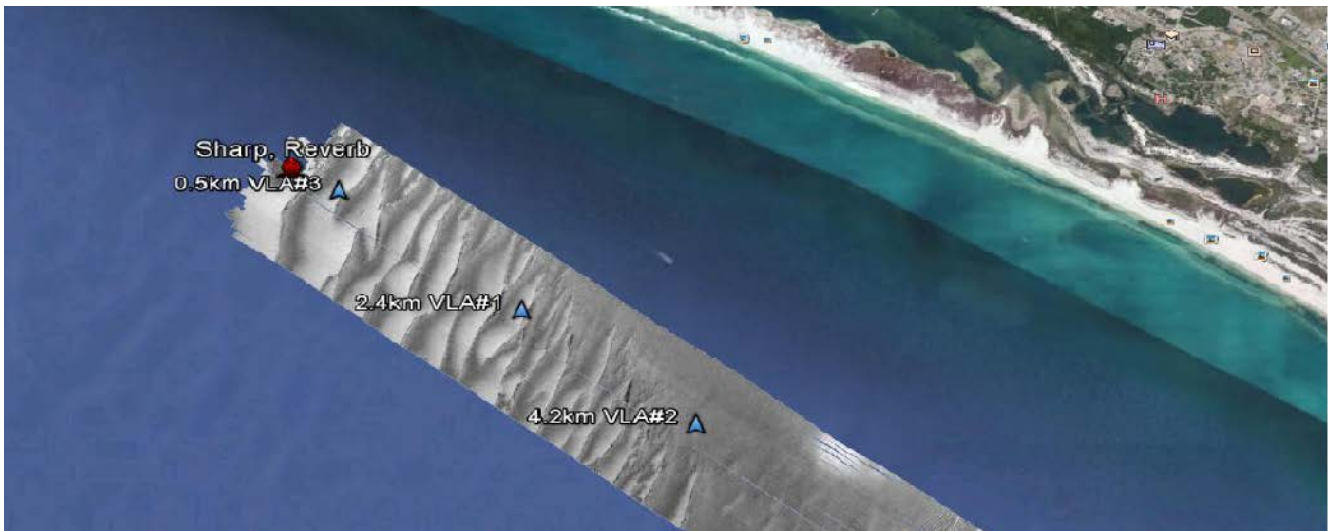
Figure 2. Multibeam survey map of the region containing the main TREX13 reverberation track showing ridge and swale structure
