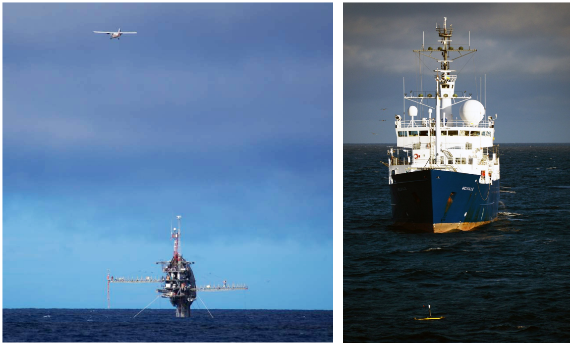
Figure 1: Measurement platforms used during SoCal2013 experiment. Left panel shows the Partenavia aircraft making a low pass over R/P FLIP. Right panel shows a wave glider (yellow object in foreground) navigating between R/V Melville and R/P FLIP.
