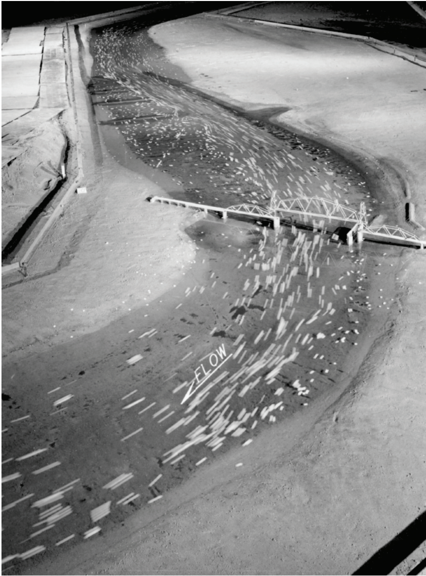
Figure 6. 1987 WES physical model study of the Jackson Bar Reach.
