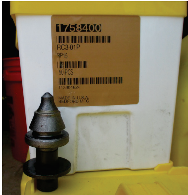
Figure 24. Wheel saw teeth, Kennametal model RP15.
