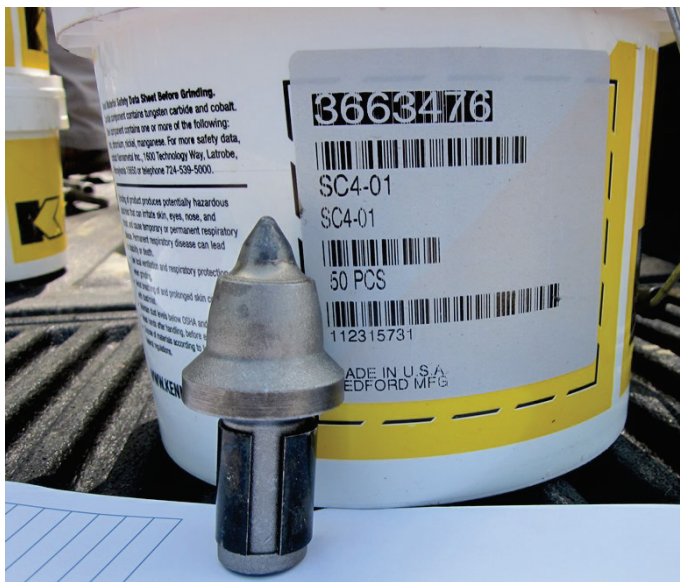
Figure 22. Wheel saw teeth, Kennametal model SM08.
