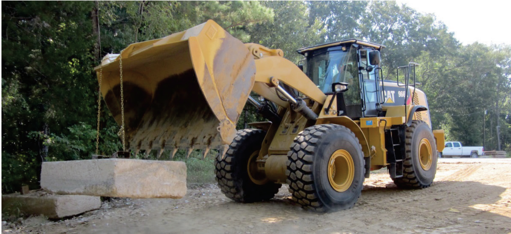
Figure 16. Caterpillar 966K front-end loader.
