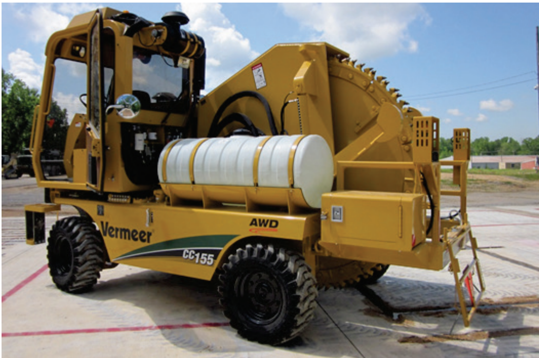
Figure 11. Vermeer CC155 concrete cutter with CC1531 wheel.
