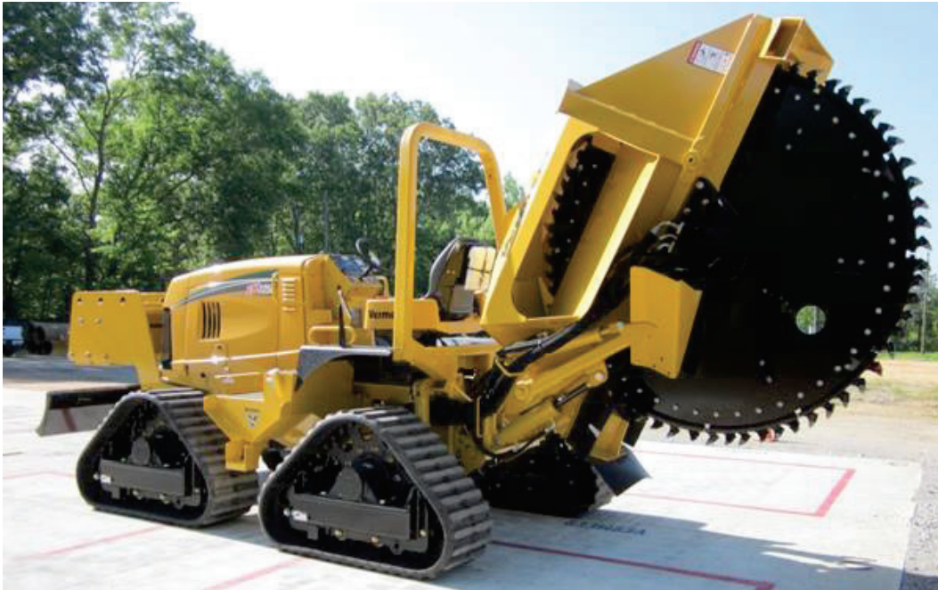
Figure 12. RTX1250 tractor with RW1236W rockwheel attachment.
