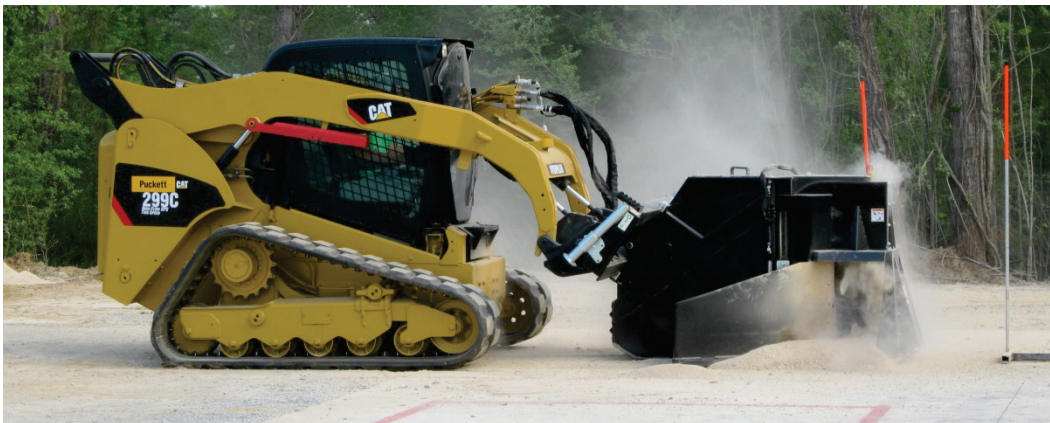
Figure 4. Caterpillar 299C CTL, operating the SW45 wheel saw attachment.
