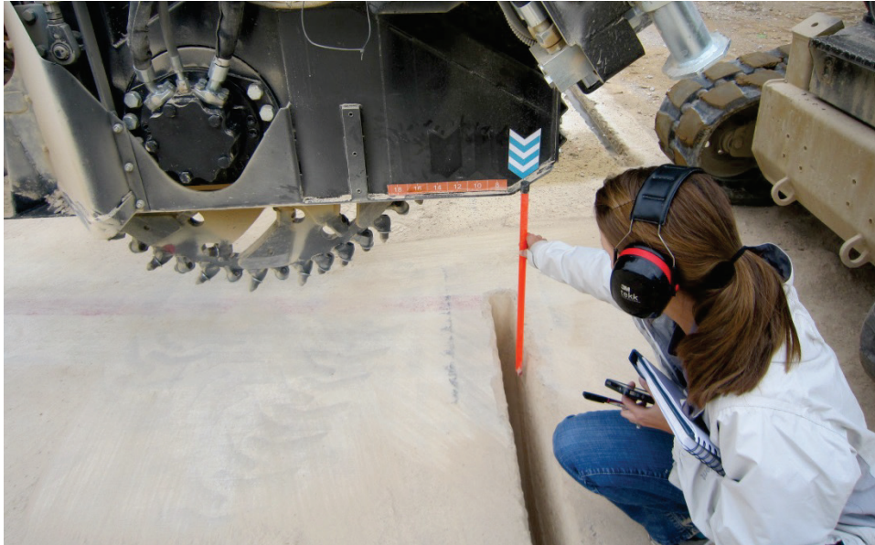
Figure 10. Using the rookie stick to line up to the edge of the crater.
