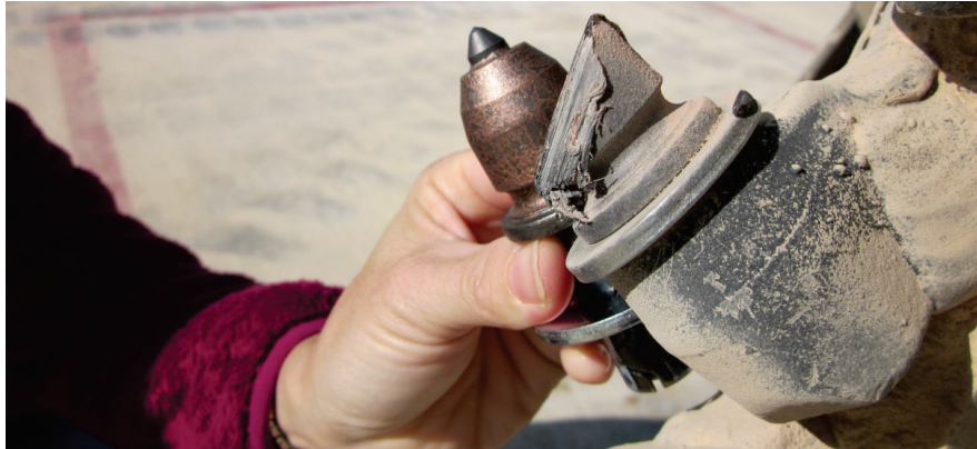
Figure 27. Worn concrete teeth after cutting, CAT model 227-7340.
