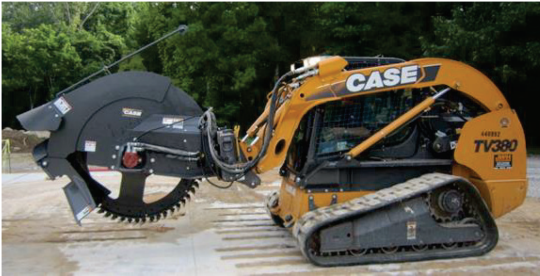
Figure 13. CASE TV380 with Bradco RS24 rock saw attachment.
