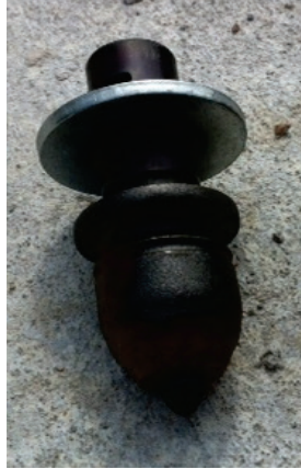
Figure 21. Wheel saw teeth, CAT model 227-7340.
