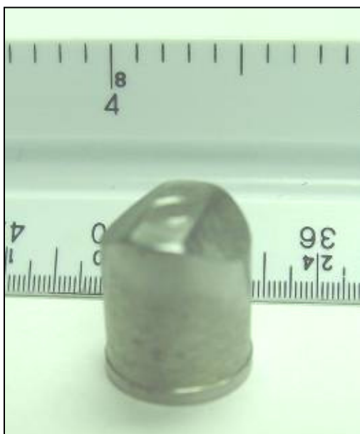
Figure 1. A 0.50 in. fragment simulating projectile (FSP), showing the tapered edges of the strike face.
