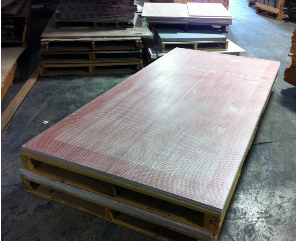
Figure 50. 2 GFRP panels with self-healing agent.
