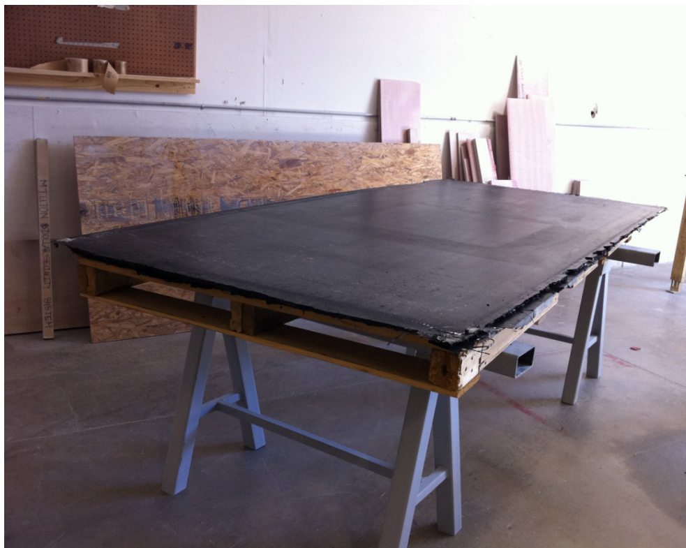
Figure 51. One of the two GFRP panels that were reinforced with CNTs.
