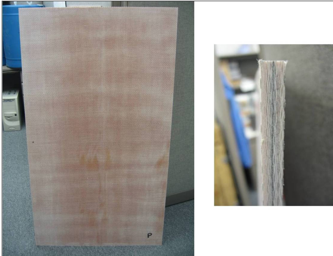
Figure 46. Polyester GFRP panel (32 x56 in.) with carbon coating incorporated (left); cross-section view of panel showing continuous carbon coating integrated with the GFRP at the middle of the panel (right).
