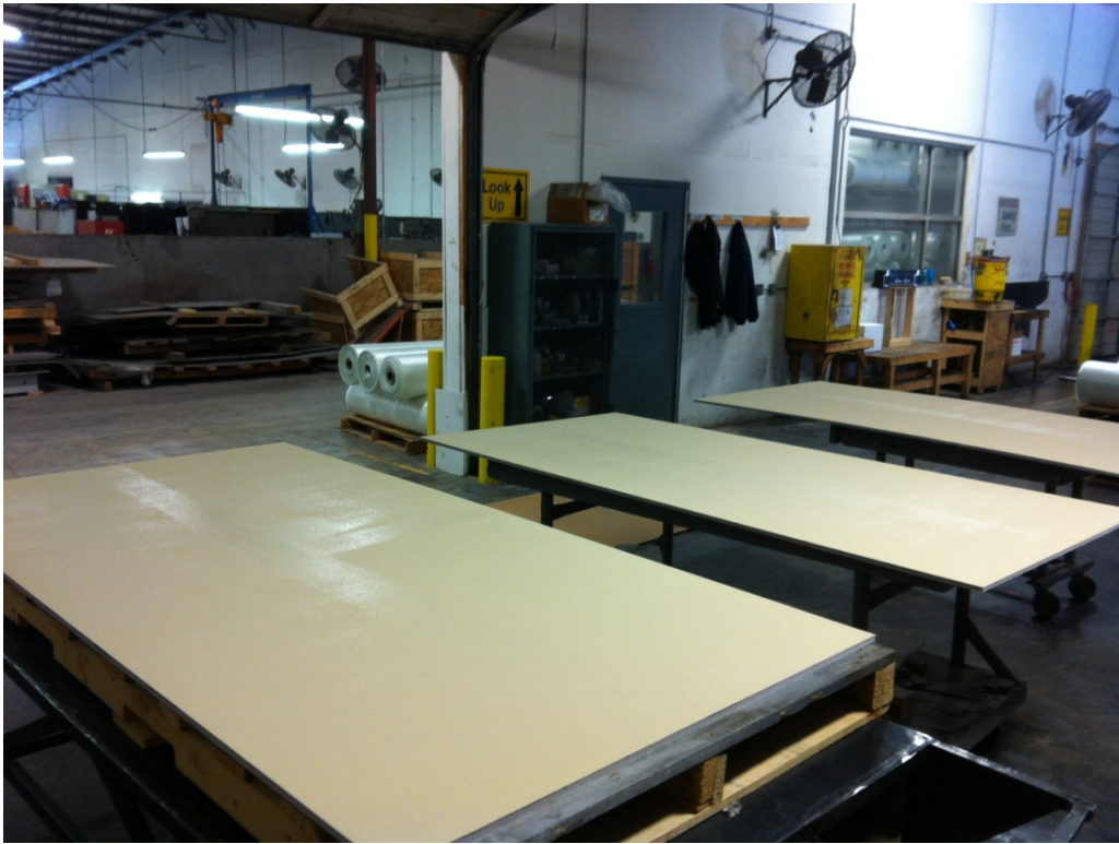
Figure 52. One panel reinforced with CNTs (left) and two panels coated with SDS coating (middle and right).
