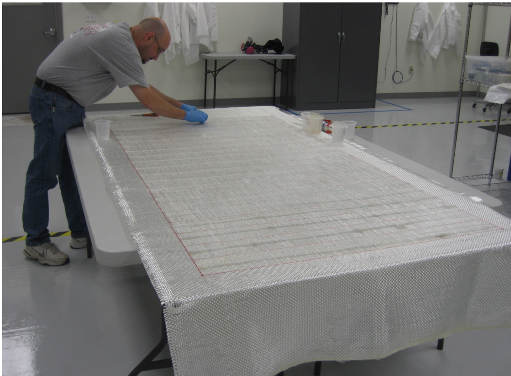
Figure 49. Placing HGFs filled with self-healing agent and catalyst on a 4 x 8 ft panel of glass fiber fabric.
