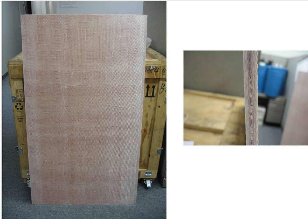
Figure 43. Polyester GFRP panel (32 x56 in.) incorporating copper mesh screen (left), and cross-section showing copper mesh screen in middle of panel (right).
