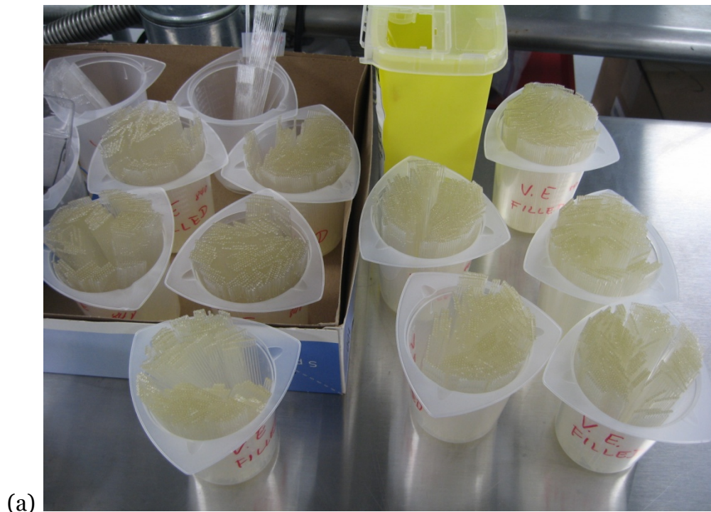
Figure 47. Groups of HGFs were prepared in three steps: (a) filled with self-healing agent; (b) filled with catalyst; and (c) filled with self-healing agent and catalyst.
