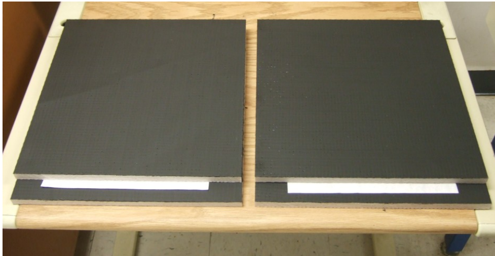
Figure 38. GFRP panels coated with MIL-PRF-85582D primer.
