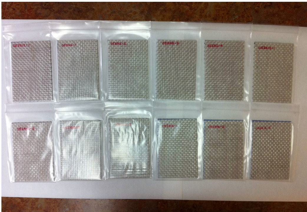
Figure 32. Baseline GFRP sample specimens without self-healing agent.
