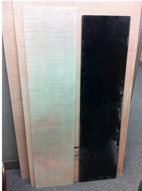
Figure 8. E-glass/polyester GFRP panels without (left) and with (right) CNT-COOH (1.0%) reinforcement.
