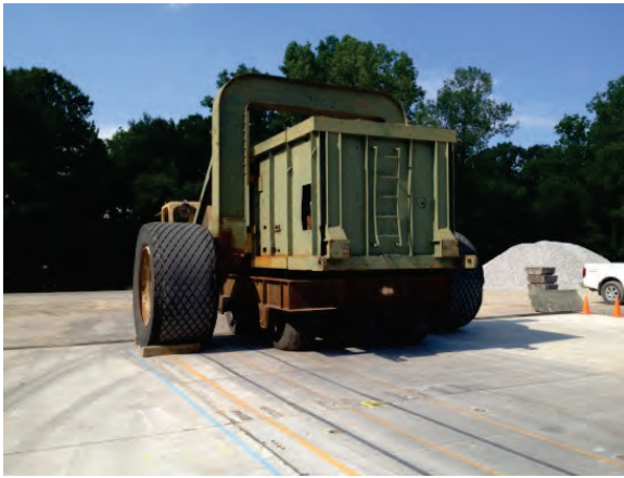
Figure 4.3. (a) C-17 load cart, (b) gear configuration, and (c) C-17 traffic pattern.
