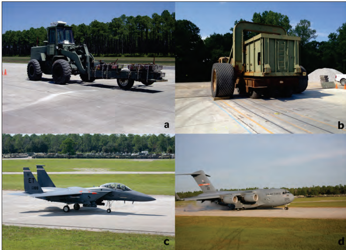
Figure 6.6. (a) F-15 load cart, (b) C-17 load cart, (c) F-15 aircraft, and (d) C-17 aircraft.
