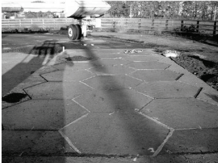
Figure A.10. Accelerated pavement testing of hexagonal slabs in France (Kohler et al. 2007).
