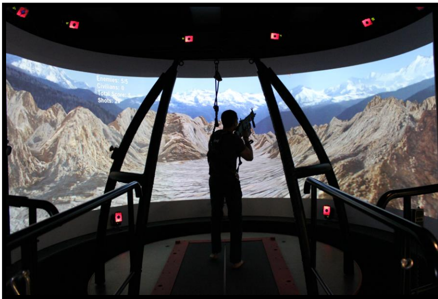
Figure 6. Example of subject walking in the CAREN system with a simulated weapon during cordite scent release.
